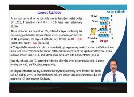
So, like your sodium like your lithium-ion batteries, sodium ion battery is also have this kind of layered cathode. So, one of the example is sodium transition metal oxide T stands for that O 2. So, there is a typical layer structure as you can see A B C, A B C kind of stacking that is there.
