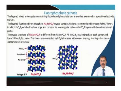
Fluorophosphate is another cathode that is being talked about. The layered mixed anion system contains fluoride and phosphate ions that are widely examined as positive electrodes for SIBs. Lot of papers have been published. This layered fluorinated iron phosphate that contains sodium ion accommodated between Fe P O 4 F layers.
