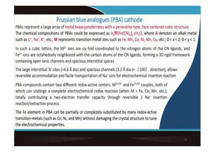
Prussian blue analogues that cathode also is very easy to make. And this basically represents a array of metal hexacyanoferrates. This is having a perovskite structure with face centered cubic lattice. Chemical composition of PBAs you can express like this. So, z molecule of water is also embedded here.
