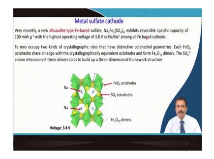
Then let us talk about metal sulfate cathodes. And this is very recent type of work alluaudite-type Fe-based sulfate sodium 2 Fe 2 SO 4 whole 3 that exhibits a reversible capacity about 100 milliampere hour per gram with the highest operating voltage is quite large here 3.8 volt versus sodium.
