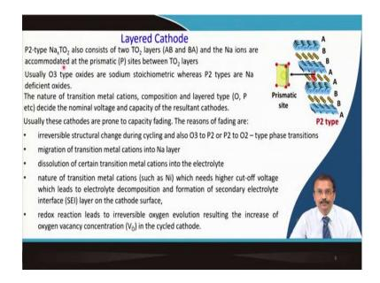
Now, this P 2 type structure of the layered material that also consists of two TO 2 layers one is AB and then BA, AB and BA type. And sodium ions are accommodated in a prismatic site between TO 2 layers. So, in between, this it is not octahedral, but prismatic layer.
