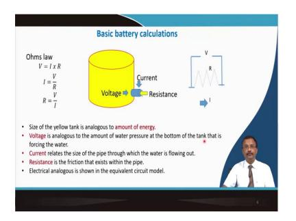
So, we can have some basic battery calculation based on Ohms law. All of you know that V equal to I into R. So, I can calculate I that is V by R. And I can calculate the resistance of the battery which is V by I. So, you can see this yellow tank that is analog analogous to the amount of energy that the battery stores.
