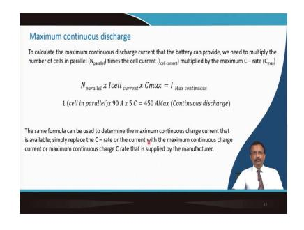
$N_{parallel} \ x \ I_{cell \ current} \ x \ C_{max} = I_{max \ continuous}$
