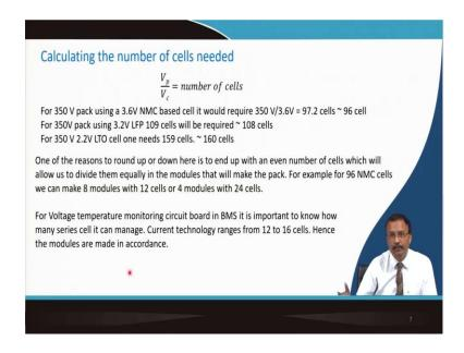
Now, it is important for you to calculate the number of cells that is needed. So, let us assume this V p is the pack voltage, and V c that is the voltage of individual cell. So, pack voltage and individual cell voltage, if you divide this then you will get number of cells.
