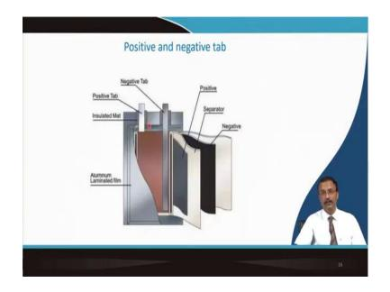
So finally, now this is a pouch cell typical pouch cell. So, instead of winding the jelly roll, here the stacking is done between your positive electrodes separator and negative electrode. And, then in order to take the connection out from the electrode you need to spot weld, this metal part which is known as tap.
