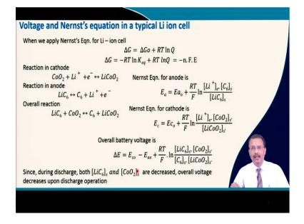
Now, it is quite straightforward to relate the voltage and Nernst equation in a typical lithium ion cell. So, when for example, we apply the Nernst equation in lithium ion cell, again we can write the free energy change that is equal to free energy change or standard condition and this term RT ln Q.
