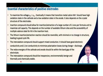
So, as you understand, if you want to maximize the voltage of course, the chemical potential of cathode must be higher than anode. So, that means, the transition metal cation for example, if you take Mn plus, it should have higher oxidation state in the cathode and if it is used in anode, it should have lower oxidation state. It also suddenly depends on the crystal structure.
