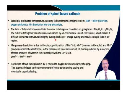
So, this is already explained earlier that what is the spinel based cathodes problem. So, at elevated temperature capacity fading that remains a major problem. Jahn-Teller distortion is also another, oxygen deficiency, manganese dissolution into the electrolyte.
