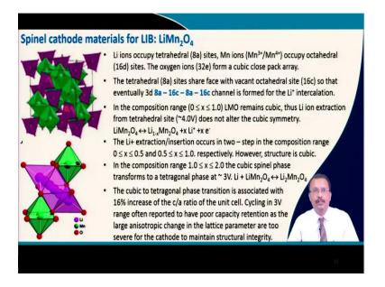
Spinel based cathode material. So, I have already explained it earlier. So, lithium ion they occupies 8a sites and manganese occupy the octahedral site and oxygen is 32e (Refer Time: 37:19) of notations that site and oxygen forms a close pack array. Tetrahedral sites are face shared with vacant octahedral site which I have denoted with 16c.
