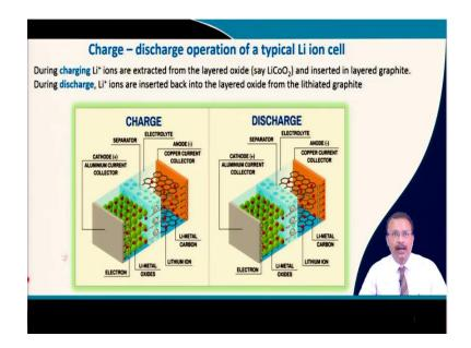
So, the operation by this time is well understood. So, we have a charge operation and during charge lithium ions, they are extracted from your cathode material say layered cathode materials like lithium cobalt oxide and they pass through this porous separator and insert into the layered another layered graphite material. During discharge, lithium ions are inserted back into the layered oxide from lithiated graphite.
