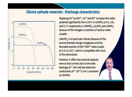
So, there are various types of olivine material. So, if you replace iron 2 plus by manganese 2 plus, cobalt 2 plus also can be replaced or nickel 2 plus that basically increases the redox potential. So, iron is somewhere here around 3.5. If it is here, then it is increased, it is increased further here, but the capacity also falls down. So, the energy density that is to be seen that how much energy density which is a product of the voltage and capacity that exactly you gain.
