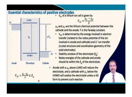
So, again, the essential characteristics as you can now understand that the chemical potential of anode and chemical potential of cathode, they are important the in case of getting a higher open circuit voltage and here F is the Faraday constant. So, this relation between the open circuit potential and the chemical potential of lithium in cathode and anode that has been described earlier as well.
