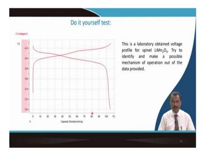
So, I have given a typical charge discharge profile of lithium manganese oxide a well known spinel. So, you can try to identify based on the lecture that we had so, far we are discussing, you can try to identify and make a possible mechanism of operations. So, what is happening during charging up to this? What is happening in this plateau and during discharge what is happening here, and what is also happening here and what is happening here?
