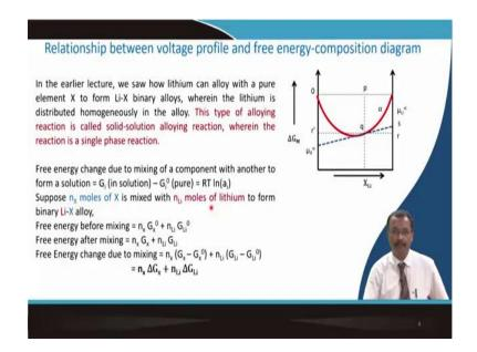
So, in earlier lecture, we saw how lithium can alloy with pure element X. So, as I told in here, I have defined the left part as X to form a lithium X binary alloys, wherein the lithium distributed homogeneously in the alloy. So, remember the diagram that I showed where lithium and this X component and sometimes I define as a. So, they are homogeneously distributed.
