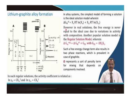
In case of lithium graphite alloy formation the simplest model that forming a solution that is the ideal solution that I described this relation this is a bit modified. So, in real solution the free energy is never equal to the ideal case due to the variation in the activity with the composition.
