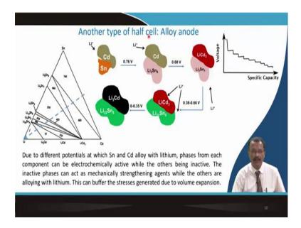
Another example can be shown where it is a ternary kind of phase system. So, this is already I have explained how it forms. So, if you have lithium alloying across this line, then for tin cadmium this binary alloy lithium will progressively form various types of alloying initially it will start to form with this cadmium will remain like this. And, then another voltage which you can calculate back this two will form.
