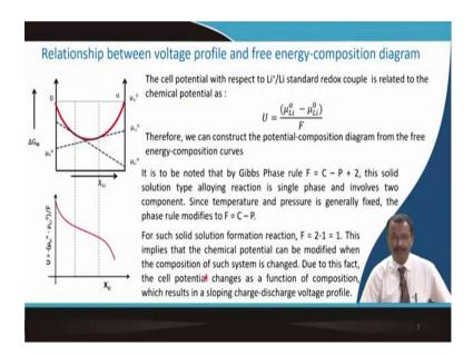
So, the cell potential with respect to lithium redox couple is standard redox couple is related to chemical potential and this already we have talked about several times this relation. So, your lithium is here for this particular composition if you take, then draw a tangent here. And, for pure lithium it is in this state, in this state.
