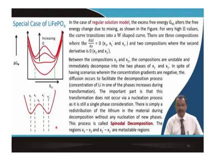
A special case is lithium iron phosphate where this regular solution model is prevalent then the ideal solution model. We talked about the excess free energy term this alters the free energy change due to mixing so, as shown in the figure. So, this term when this omega term increases, then from regular this type of bold type of free energy diagram as you increase this delta term, you see that slowly it goes to a 2 minima condition.
