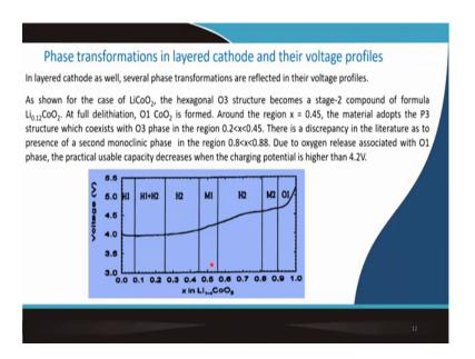
So, phase transformation already I defined in case of lithium cobalt oxide several phase transformation that is possible. So, in case lithium cobalt oxide hexagonal O3 structure becomes a stage-2 compound with formula of typical formula of Li 0.12 Cobalt Oxide. At full delithiation, O1 type of cobalt oxide formed. Around the region x equal to 0.45 the material adopts a P3 structure.
