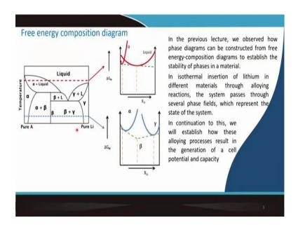
So, we will start with again the free energy composition diagram and the phase diagram of a binary component system, one is a pure component which is defined as A, and another side is pure lithium. So, sometimes in some of my slide instead of A I put X and the right hand side is always lithium. So, lithium content increases here and it forms various types of solid solution and mixture of solid solution.
