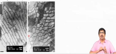
And this kinds of dislocation where you can see that it forms its own substructures and the size of the substructure is within the nano meter scale and the mis orientation between them is less than 1 degree. So this mosaic structure concept is very much valid even today and we can think of that this dislocations of structure is basically is a replacement earlier mosaic structure that people have imagined and they try to explain the effect of string one size broadened.
