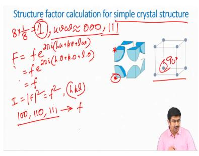
Now, let us forget all of this and let us start doing some simple very simple and fun things, calculation of structure factor for various types of crystal system. So, this is a simple crystal structure. So, simple crystal structures, how do we define a simple crystal structure? Basically, a simple crystal structure has, if we consider something like an orthogonal crystal system. That means this angles we imagine that all of these angles are 90 degrees.
