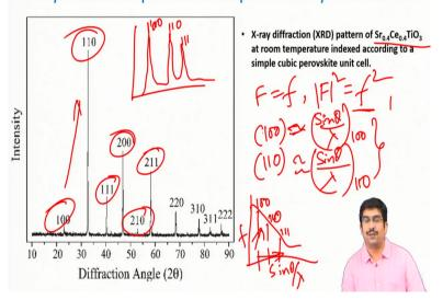
X-Ray Diffraction pattern of simple cubic crystal structure
