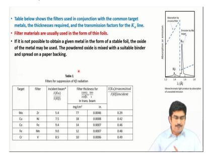
So, if it is, I think the relationship goes if I am not wrong yes, its copper and nickel. So, if nickel is there if the target is copper, I can use a nickel filter.
