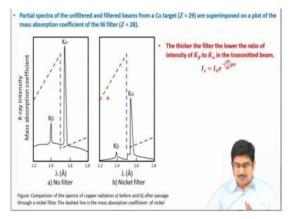
The most the most important example here; so, if I have a copper 29 as the target metal, I will be using a nickel filter 28 atomic number as the filter material. So, now what happens is if I think of about this then what this filter material does is it will absorb the K beta component because what is happening is if we can we can think of this one basically. So, we have the K alpha and K beta radiation coming out of copper.
