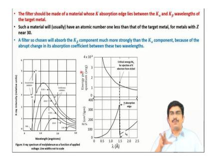
So, that is where these x-ray filters the concept of x-ray filter comes in. So, we can use basically a filter to separate out the K alpha and K beta primarily. Of course, so the filter and here we will take the advantage of x-ray absorption. We understood that x-ray absorption also is very much specific; it happens at a specific wavelength. So, that also we have seen and it is related to the characteristic radiation only.
