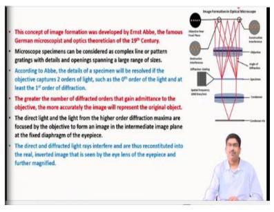
And this is how the image formation happens in the real plane in somewhere over here, in the image plane this is how the image forms in case of an optical microscope. And little later we will come to know that this method of forming the image is called bright field image generally. Now, this entire concept of image formation is basically credited to one person called Ernst Abbe.
