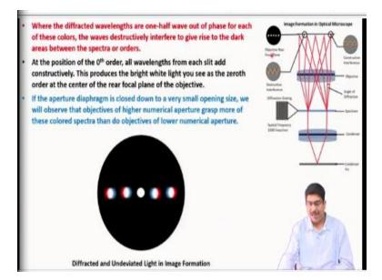
Then the next thing that happens is that when it diffracted wavelengths are exactly out of phase. And if you just able to understand that this is one diffraction, this is happening from one of the diffraction grating and the sample has many, many such diffraction grating. So, this kind of blue and  $1^{st}$  order diffracted beam,  $2^{nd}$  order diffracted beam, direct beam they are forming for each of these diffraction patterns.
