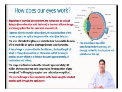
So, the first thing we must understand before we progress with any kind of microscopy, in particular optical microscopy. That we have to understand how our human eye basically works. So, our human eye works in the same principle as an possibly an optical microscope work out. For that matter any kind of phones, digital phones these days digital cameras these days either in your cell phone or the digital camera that you use to capture some photographs.
