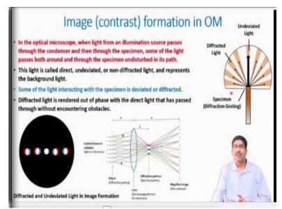
Now let us discuss how the image formation happens in an optical microscope. So, in the optical microscope, what happens is that when the light passes through, let us say that this is an specimen which is kept here, the light falls over it. And some part of the light or maximum part
