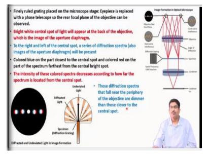
Now, in order to really verify that, this is the mechanism of image formation, what we can do? We can do a simple experiment and we can bring something called a diffraction grating, which is nothing but an specimen having a very regular pattern onto it, very regular openings onto it diffraction, that is called diffraction grating. So, this diffraction grating when we brought here, then what we will be getting is this kind.
