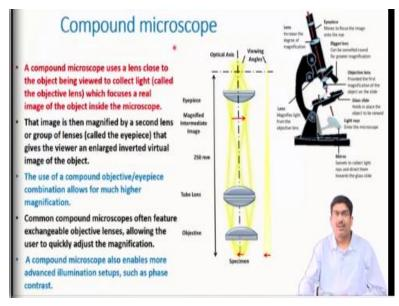
So, compound microscopes, again this is possibly what we have seen in your school, in +2, this is a fine example of that compound microscope where you have one set of lens which is called usually the objective lenses. And objective lenses, what does it do? It basically so you have a lens you have a source, usually as the mirror that and if you use the light as sunlight, that is what we generally do our good old days, that is how compound microscopes used to be.
