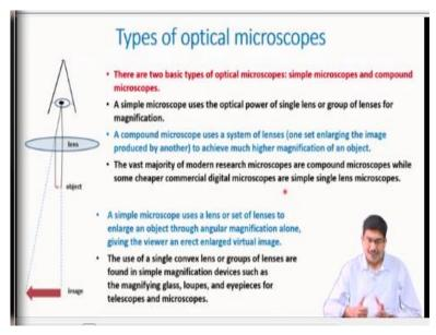
So, these are the ways the images are formed. And as I just said now say there are 2 basic types of optical microscopes. One you can call a simple microscope and another one is a compound microscope. Simple microscope, as the name suggests you just have usually one single lens like a magnifying glass or you can have multiple lens also, if you want to just improve the magnification you tend to have a little bit more complex system and bit more complex lens system more than one lens.
