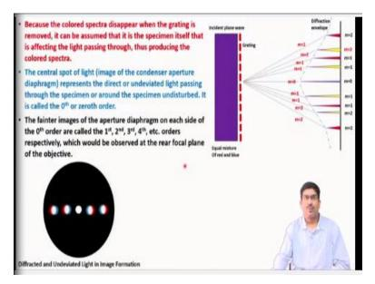
So, why this is happening? As I said this is a diffraction grating that you have the central beam or the undeviated direct beam that is passing through that is called the zeroth order beam. And the other ones are basically called the first one is called a first order diffracted beam, then you have the second order diffracted beam and so on and so forth. That depends on the order of diffraction; we are not going into that when we discuss about the diffraction phenomena.
