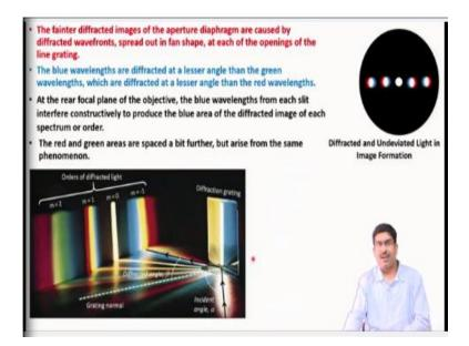
Now what happens is that when the diffraction grating is placed there and the diffraction phenomena happens through this diffraction grating one, single one of them. Depending on the wavelength, so this diffraction phenomena is very, very sensitive to the wavelength. And the wavelength in a white light what we are considering the direct light which is white light and that white light is now that is divided between these various colours depending on their wavelength.
