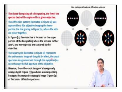
The another point that is diffraction or phenomena on the diffracted beams is related to the specimen features, in order to prove that we can just look at 2 other things. First of all we can check out this kind of a diffraction grating in which there is a difference between the distances of these diffraction gratings from which the diffraction phenomena is happening. And what we can observe is that the closure the spacing of this line grating, so these are called line gratings.
