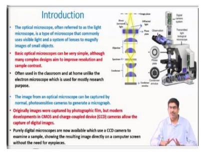
So, the optical microscopes sometimes also referred to as the light microscope. And this is because it generally uses light, visible light as a source of signal. And remember what I said about source of signal and then detection signal and the way of detection. So, in this case the source of signal is basically light, that is why it is called a light microscope. And in this truer sense, the optical microscopes are very, very simple.
