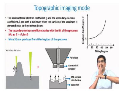
Now how this topographic imaging mode basically works? So, the backscattered electron coefficient eta and secondary electron coefficient delta both of them are minimum where the surface of the specimen is perpendicular to the electron beam. So, if you imagine this is a secondary electron mode and imagine that this is exactly representing this, but we are now seeing instead of a top view we are seeing a side view of this specimen just imagine that.
