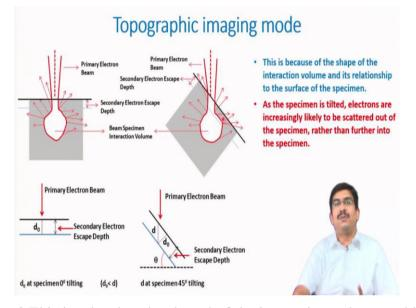
Now why is it so? This is related to the shaped of the interaction volume and its relationship with the surface of the specimen. So, if the beam is directly falling over this specimen surface or the beam is falling at an angle with the specimen surface the shape of the interaction volume does not change. It always remains of this shape and always is beneath this beam directly.
