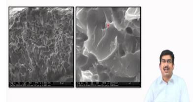
Topographic imaging again very interesting example already I said that the SE signals or SEM is very much used for studying the fracture surface and for fracture surface of course it is completely in topographic mode. So, you see it this is a single phase material and the topographic imaging here is giving the contrast because of the difference in surface roughness.
