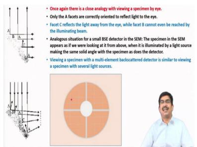
And this we can do it with this multi component detector so you know this multi element detector backscattered detector when I was discussing I said that there are four different detector and you may be wonder why we are creating four different detectors we could have only single detector here. This is because the backscattered detectors are such that their topographic contrast they are sensitive.
