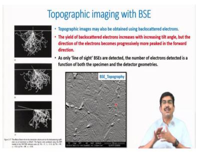
So, with this we will be moving to topographic imaging with BSE and topographic as we said topographic images can also be captured in BSE mode just like in SE mode. Here also the same thing when we tilt the specimen the shape of the interaction volume does not change. So, in this case that is the Monte Carlo simulation again shown here instead of specimen tilting what we can imagine that the beam itself is tilted basically by the same thing.
