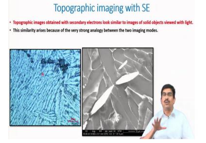
So, topographic imaging of SE also one more point very important is that it looks pretty similar to the image viewed with light. So, if I compare this is a light microscopy image from the same titanium alloy, alpha beta titanium allow this is the light edge so filter is used forget about that, but it is basically giving almost the same kind of contrast. Here also the two phases the very distinctly appearing.
