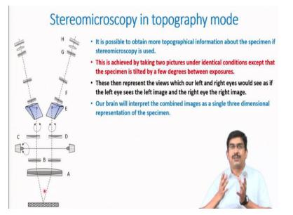
One more very important application of this topographic mode or secondary electron image usually it is done in secondary electron image is called the stereo microscopy. Now what is stereomicroscopy? Here very briefly we discussed about stereomicroscopy. So, what stereomicroscopy does is pretty much the same way we see images with our own eye the way we see images like for example our human eye we have two eyes.
