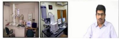
So, from here we will just quickly start the discussion on chemical analysis in electron microscope. So, in electron microscope the chemical analysis can be done in two different ways. Basically, either we can measure the wavelength that is called wavelength dispersive spectroscopy or the energy of the X-ray signal characteristic extra signal which is called the energy dispersive spectroscopy.
