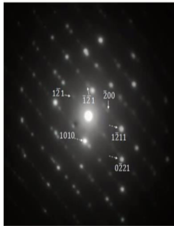
Spot diffraction pattern of forged Ti-6Al-4V alloy. Two phases are observed in the pattern, namely, \alpha and \beta with Z = [1\bar{2}1\bar{6}] and Z = [012] , respectively.
