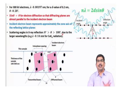
Now let us put some typical numbers. Let us throw some typical numbers in this Braggs law and try to find out what is so special about electron diffraction, how this equation gives us an idea about electron diffraction. So, for let us say a 300 kV electron which is very typical that we use for a TEM instrument. Lambda we know the relationship between accelerating voltage and wavelength.
