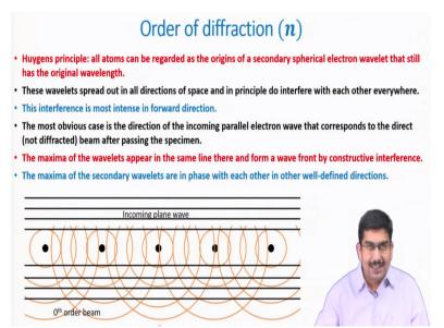
Now another thing that we need to understand here is the order of diffraction we will go one by one. So, this order of diffraction is basically that n in the Braggs now n lambda equals 2 d sin theta so what is that n here. In order to understand that I found there are many ways we can understand, I found the best way to understand this is by going this one called Huygens principle.
