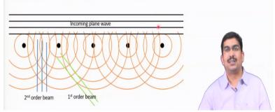
So, now let us see this. So, in the first case what we can imagine is that along this direction the one given with this green color. So, in that direction what is happening is that the first maxima from the first atom the first maxima of first atom is coinciding with the second maxima of the second atom and the third maximum of the third atom and so on and so forth. So, if we imagine this is the first one.
