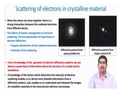
So, the scattering of electrons when this happens the constructive interference along certain direction happens then what it produce is a very regular variation of intensity, we have already seen it for amorphous material even for them the intensity variation with scattering angle they are diffuse maxima and in this case in crystalline material these are much more prominent.
