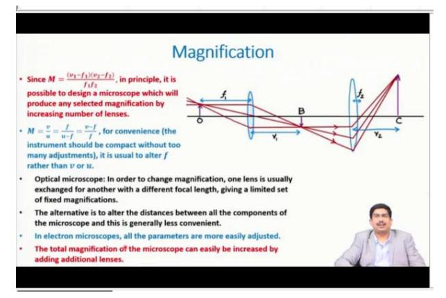
So, the next one is magnification and just now we discussed that in magnification using a lens combination the maximum magnification that we can have is this much. So, what happens is that if you see this magnification which is obviously expressed by the image distance by the object distance and also the magnification you can express it in this way from the thin lens equation.
