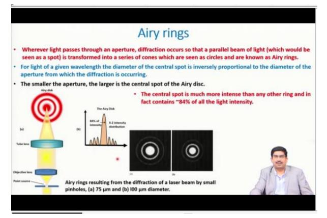
And that is what is shown here that, when the light passes through any small opening and in this case, the small opening you can consider that as the apertures that is used along with this either condenser lens system or objective lens system, the apertures which are used that can you can consider them as this very small opening. So, when this parallel beam of light which is otherwise should be seen as a central justice spot.
