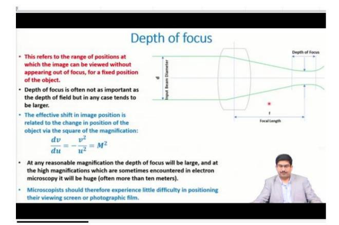
The similar term is depth of focus. So, this is what the depth of field I am sorry. This is what the depth of field and another point is depth of focus. So, depth of focus is something to do with the image side. That means it is dealing with the distance within which the image plane. The image can be move and still appear in focus. For the same object distance without moving the object how much I can move the image plane so that they will still appear in focus.
