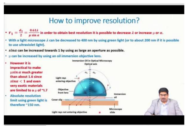
So, how to improve resolution from the concept of numerical aperture and this relationship that just now we have discussed. So, how we can improve resolution of any microscopy system is that is what we want, basically. So, in order to achieve, maximum resolution, we have 2 options. Either we can decrease lambda or we can increase mu or alpha here from this.
