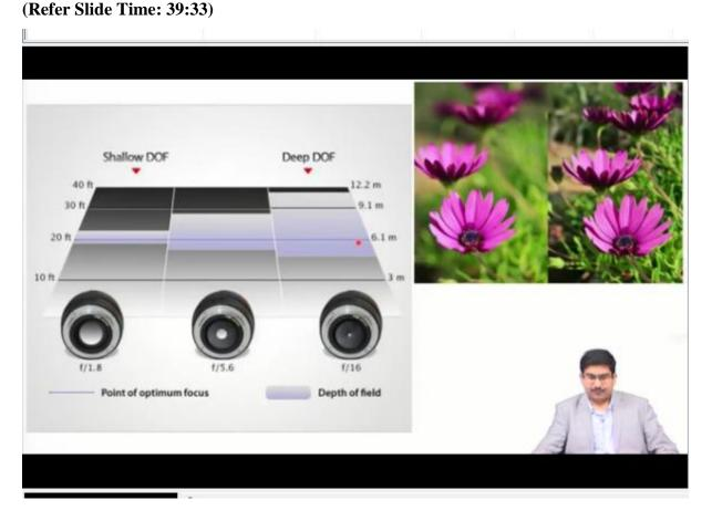
So, here also again, the same thing is shown the relationship between the numerical aperture and the resolution. So, as you can understand that numerical aperture if I have a smaller numerical aperture, then that means smaller numerical aperture means smaller  $\alpha$  value, the semi angle for this any aperture system if I have it smaller, then I can improve even not only resolution I can improve the depth of field here.
