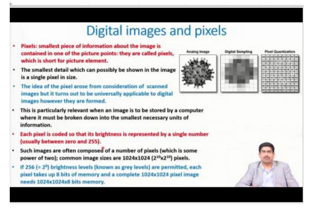
One more important point that we can possibly discuss here is the digital images and pixels. And basically digital images these days all microscopy systems are taking images and as a digital image. So, in a digital image, what do you do, this is an analog system or analog image and you correspondingly you create a digital image, digital sampling. Digital images are basically characterized by something called pixels, which is a short form of picture elements.
