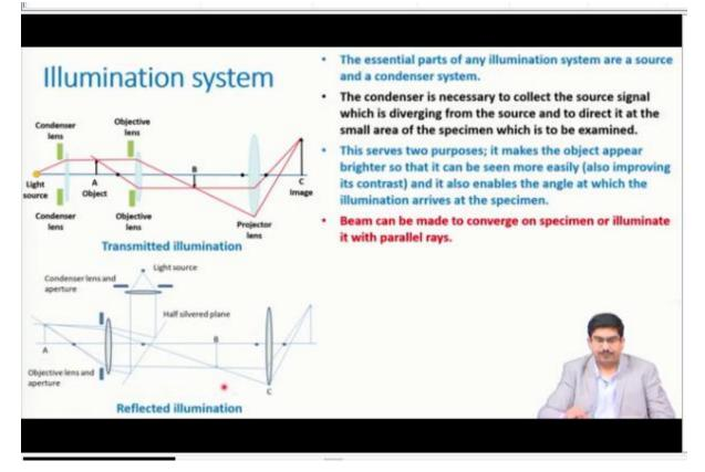
So, again, if we look at the illumination systems the illumination system typically they contains a light source and a condenser system and basically the condenser system is our condenser lens or condenser system and typically what it contains is a lens plus an aperture. So, any kind of lens you see basically condenser lens and objective lens that comes with an aperture system. So, together they formed this condenser system and objective lens system.
