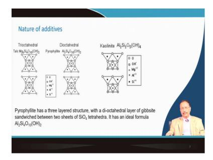
So, the pyrophyllite as you can see it has a three-layer structure. So, one is a dioctahedral layer of gibbsite, it is based on aluminium hydroxide which is sandwiched between silicon oxygen tetrahedra and ideal formula this is given by this Al2  $Si_4O_{10}(OH)_2$ . So, this can be used along with the clay which is kaolinite, in the tile composition to make a dry pressed article.
