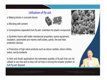
So, it is a problem to utilize it, but people have started to utilize it and making brick by mixing it with cement and sprinkle water and press it and then sprinkle water so, that the cement gets strength. So, that is a known technology and brick and concrete blocks that is that has been used part of it is also used during cement production. So, that is the known use of fly ash.
