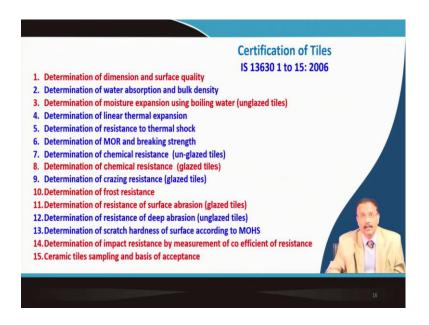
So, once the fly ash base tiles are made, then there are about 15 tests that you will have to do. First the dimension quality absorption of water, absorption of moisture, then linear thermal expansion coefficient, resistance to thermal shock modulus of rupture which tells the strength, chemical resistance both in glazed and unglazed condition then the frost resistance which is not very important for our purpose surface abrasion.
