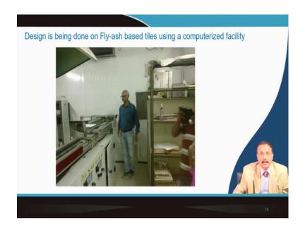
So, the tile is something like a paper and any kind of design you can make out of this computer type printer and on the glaze surface on the glaze surface it will print the design that you want on the tile surface.
