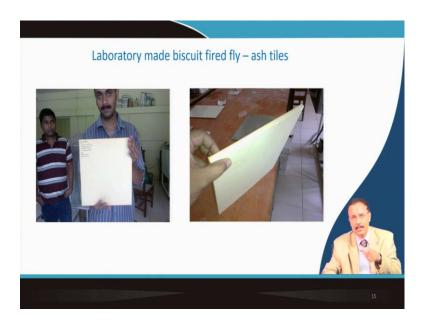
So, this is the flat tile that can be made in the laboratory which is uniform in thickness and quite big in shape we are testing small samples, but the optimized parameter it is sufficient to make a large tile these are not coated it is not glazed. So, call it is a biscuit fired tile made out of fly ash.
