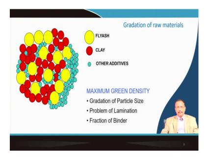
So, you can see that you have fly ash which is having this large particle, and you have will have to judiciously select the particles of clay they are usually spherical in nature, spherical in size and other additives like pyrophyllite or red mud.
