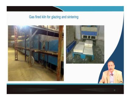
And then finally, it will have to be sintered at high temperature. So, instead of a small furnace, you have a tunnel kiln very large furnace where this biscuit fired and glazed material will go in and they will undergo at different temperature regime so, that eventually the glass will form and here the thermal expansion mismatch is a very critical parameter.
