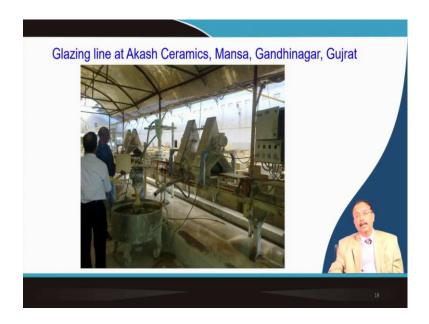
So, before that we need to glaze it. So, glaze as I told that fly that this tiles need to be glazed because intrinsic porosity is quite high for this type of fly ash this thing about 14 percent porosity is there. For all practical purpose you do not allow the porous ceramic. So, you will have to make a glass layer we call it glaze.
