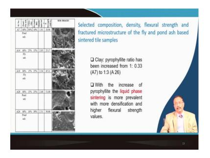
And you optimize certain composition of the fly ash, clay, pyrophyllite and look at its microstructure at different stages and different compositions and finally, you select that which one is good in terms of the mechanical properties.
