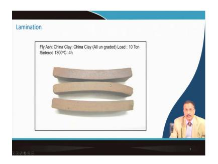
So, the lamination is something similar to this, you can see that after sintering the sample that was made out of this fly ash they just bent like this. So, gradation was not done for this samples. So, the finer particle they were floated on top during pressing and after sintering they are laminated.
