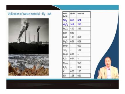
Fly ash is a problem in India, where most of the electricity that is generated out of coal. So, coal is burnt to boil water and steam is used to rotate the turbine blade to generate electricity. So, ashes are generated huge quantity of ashes and this ashes are actually dumped in the form of a slurry and it forms some kind of this muddy zone and this we called a pond ash.
