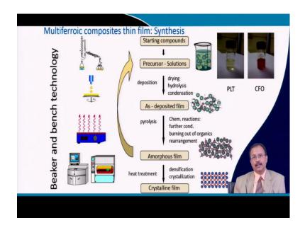
Now, for a bulk state one can make it by mixing these two things together, but it is already as I have mentioned that once you are talking about a device that you will have to make an integrated device which is integrated to silicon semiconducting silicon circuitry film. So, there it is quite important for you to grow it is in the thin film form. So, and integrate with the silicon substrate underline silicon substrate.
