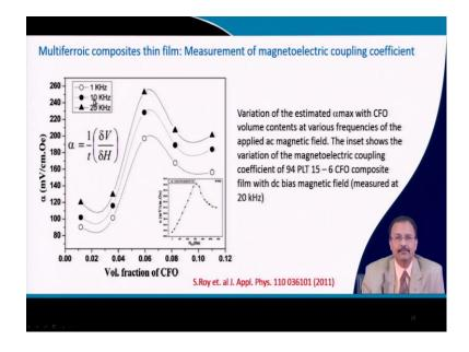
So, based on that this value of alpha that was measured, so you can change the frequency of the field that you are applying at different frequencies. And then this alpha you can measure or estimate from the measured voltage and the field the voltage and field this del V by del H and knowing the thickness of the film.
