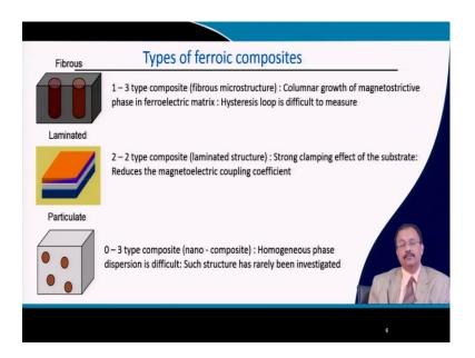
So, this distribution of one phase into the other that could be a various types and various different types of composite is possible. The three prominent examples are 1 -3 composite. So, here 1 is the dispersed phase which is in the form of a fiber as you can see
