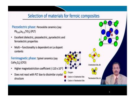
One example can be given that is ferroelectric in nature so you know that a b o three type of material particularly lead titanate is a ferroelectric is a well known ferroelectric material and it is doped with lanthanum. So, lanthanum is in plus three valence state which is replacing mostly plus two lead but it has a probability to go to titanate side also.
