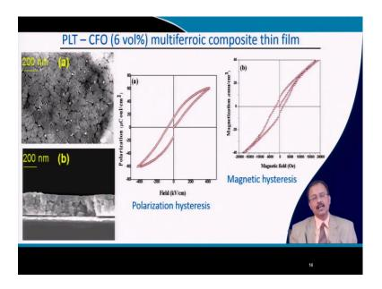
Then you would like to see that how uniform is this film. So, for that you will have to do a cross section this is the surface of the film which is analyzed by the scanning electron microscope once again. And you can see a good granular structure of lanthanum titanate and the dispersion very small dispersion and very homogeneous dispersion of cobalt iron oxide mostly along the grain boundary of this film.
