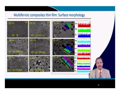
Now, if you see the actual photograph of this material. So, PLT film it is having very small grain size as you can see that and inside that this cobalt oxide grains are individually dispersed. So, for very small volume content you cannot readily identify it, but has progressively it increases from initially from 1.5 volume percent that is too small then 4 volume percent then 6 volume percent then 8 volume percent.
