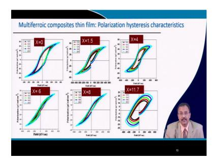
Then their hysteresis behavior also should be there. And as you can see pure material is nicely ferroelectric and already in the last lecture we talked about the ferroelectricity so they exhibit good ferroelectric loops and this each of this loop they are taken in progressively higher applied field. So, we call this is the nested hysteresis loop.
