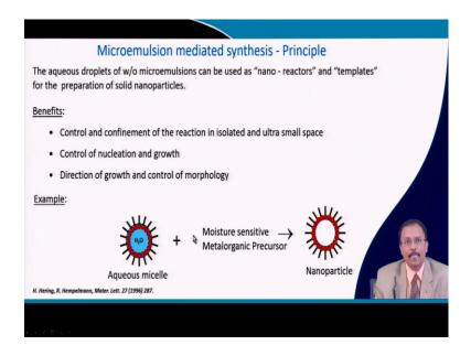
So, this concept was used this micro emulsion mediated synthesis. So, aqueous droplet water in oil, this micro emulsion that can be used as a nano reactors, and basically a template for the preparation of solid nano particle that was the idea to prepare a very small nano particles which will not scatter light. So, it will be a transparent solution, but
