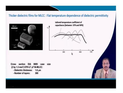
Now, this is due to the different coating layer of zirconia. The Curie temperature for each of this particle is different. So, once you do a temperature dependent dielectric measurement, then instead of a sharp dielectric maxima following the Curie transition, Curie law it is having a several of such peak and eventually it gives you a very flat kind
