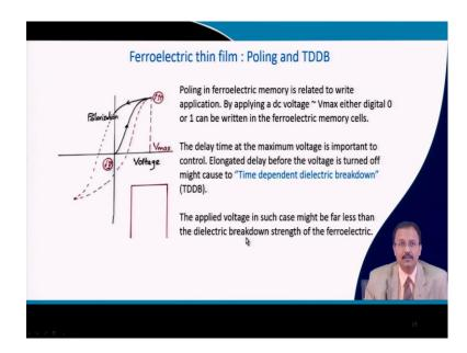
Now, in the virgin state you know that the domains are in all possible directions. So, if you apply a dc field something like that and there is a soaking period of this field, then and also this voltage is more than the cohesive voltage and very close to the maximum voltage which this film can withstand.
