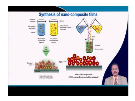
And this micro emulsion is has another effect that you can have two different types of material prepared in the same way. So, one is I have shown barium titanate here. And similarly zirconium alkoxide that can also be grown, and then they can mix together and deposit the film something like this. So, either you can deposit a single component film or you can make some kind of dopant or composite.
