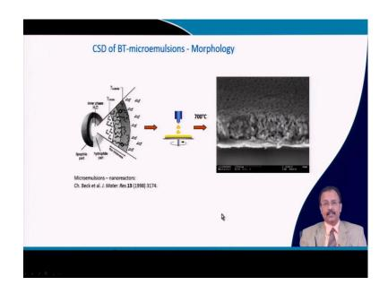
So, here it is shown that this is a core shell kind of structure, and that solution itself is spin coated and eventually annealed. So, you have a substrate, then you have metal, and then you have the thick film that is deposited there on top of it.
