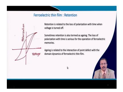
Another defect which is very important is called retention. You have written either 0 or 1 in the ferroelectric memory, and then you leave the memory as such then you will find that slowly there is a loss in the polarization. So, the polarization drops down here. Again you start to read it will start from this place instead of the original place.
