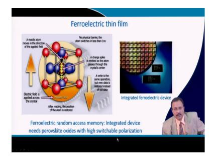
So, we will start from the perovskite crystal structure as you can see that already we have described it. So, there is a mobile cation here. So, this mobile cation moves in the direction of the applied field. So, if you have a positive field, then it if it goes up, then it is switchable. If you put a negative field, then this will be in the opposite direction, and there is no physical barrier for this kind of switches.
