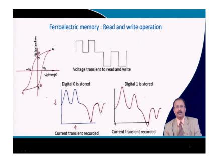
So, it is very interesting to know that how a digital 0 and digital 1 is first stored in the material that I will come later on, but more importantly what exactly is stored whether it is a digital 0 or 1 that can be identify by having this kind of voltage transient. So, as you can see the initial voltage transient is a positive up, then there is a delay here.
