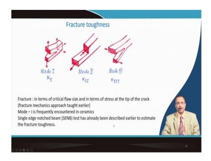
Fracture toughness already we have described earlier. And usually mode one is frequently encountered in the ceramic. And as a part of my earlier lecture already we have described that single edge notch beam test abbreviated as SENB is actually this is used to estimate the fracture toughness of the brittle ceramics.
