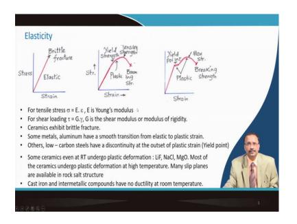
So, this is the curve which I described earlier, this is for the brittle material. And the stress and strain, this curve is linear in nature. So, stress is proportional to strain. And the proportionality constant is the elastic modulus. So, E is defined as the elastic modulus; it is termed as Young's modulus. For shear loading, shear stress is proportional to shear strain.
