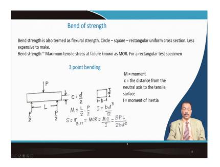
Usually, we measure the bend strength. So, this already I have described earlier. So, 3 point bending is done. Two supports are there. So, you know that this is the span length. So, first you calculate the moment, and moment of inertia.
