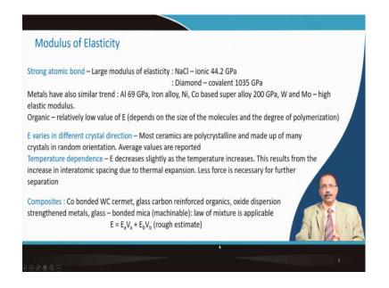
So, if you consider this modulus of elasticity, usually if it is having a strong atomic bond, then usually the modulus of elasticity is large. Sodium chloride, it is having ionic bond. So, it has elastic modulus about 44.2 Giga Pascal. Diamond is a covalent which has exorbitant elastic modulus about 1035 GPa.
