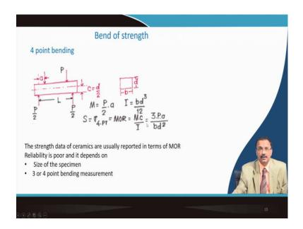
In 4 point bending test, the formula is a bit different. But here the similar kind of arrangement is made, and it depends the strength data of ceramic is usually reported in case of most of the ceramics like the MOR value – Modulus Of Rupture. So, the reliability is one factor. And the reliability depends on the size of the specimen and whether you have done either a 3 point or 4 point bending that also is important for you to accurately predict the strength value.
