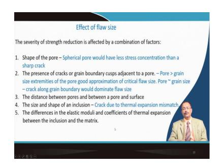
So, the severity of the strength reduction is actually affected by a combination of factor. So, pore is one of them – spherical pores that will have a less stress concentration than a very sharp crack. So, it is better to have spherical pore. The presence of crack or grain boundary adjacent to the pore, so that will affect the strength of the ceramic. The distance of the pore and pores and between the pore and surface that is also important.
