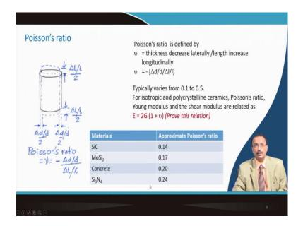
We can define Poisson ratio is basically when the sample is under tension, then it will be elongated in this direction, but it will be contracted in the lateral direction. So, Poisson ratio is the lateral deformation by longitudinal elongation. So, it varies about 0.1 to 0.5. For isotropic and poly crystalline ceramics, Poisson's ratio, Young's modulus and shear modulus they are related.
