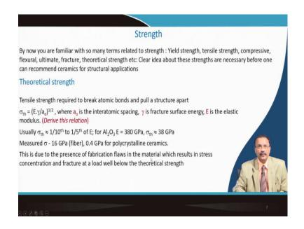
Now, by now you are familiar with so many types of strength. We talked about yield strength, we talked about tensile strength, compressive strength, flexural strength, ultimate strength, fracture strength, theoretical strength, so, so many strength we have described in our previous lecture when I talked about the mechanical properties of the non-metallic materials.
