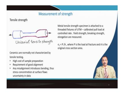
So, usually, in case of the ceramic the tensile strength is measured by making a specimen something like this, but this sample preparation is costly and very good alignment is required to make this kind of samples because any small misalignment will generate the stress concentration. So, usually unlike the metal the ceramic is not measured by this kind of sample.
