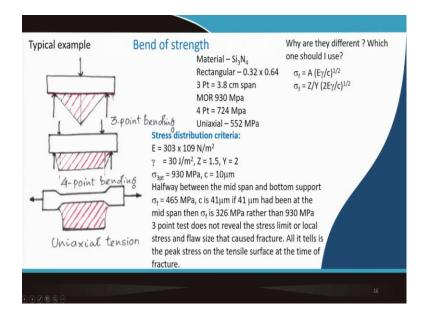
Now, this is an example. A centered material is formed in the form of silicon nitrite. It is a rectangular size 0.32 by 0.64 centimeter is the cross section. And in case of 3 point, this span was 3.8 centimeter. So, the MOR was measured as 930 Mega Pascal. If you do the same experiment in case of 4 point, the value is reduced to 724 Mega Pascal.
