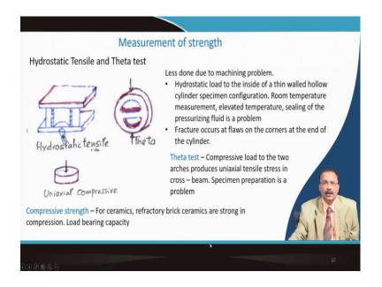
Usually that tensile sample preparation is a bit tricky, but this hydrostatic tensile strength measurement is also done, but that is also having a machining problem. So, the hydrostatic load inside the thin walled cylinder at room temperature you can measure its strength elevated temperature ceiling is important. And fracture usually occurs at the corner or at the end of the cylinder. And this is one way to measure the strength of the material.
