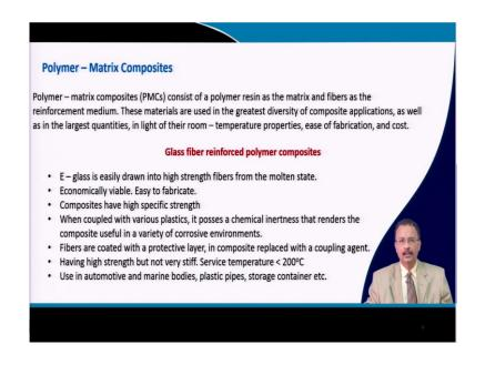
So, it will be taken in details, but here in this lecture particularly I am concentrating on polymer matrix composite. And this consists of basically a polymer resin as the matrix which are relatively softer and fibers as the reinforcing medium.
