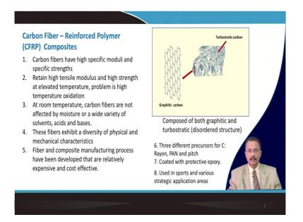
Another fiber that is used is carbon fiber and accordingly we term it as Carbon Fiber Reinforced Polymer Composite and it is abbreviated as CFRP; Carbon Fiber Reinforced Plastic Composite. So, carbon fibers they are used because they have high specific modulus and specific strength is also quite high and they retain high tensile modulus and high strength; even at high temperature.
