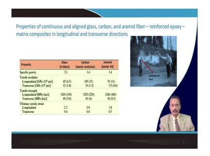
So, I have compared here three different types of fiber reinforcement; the E glass, then you have the carbon and you have the aramid fibers. And you can see their tensile modulus both in the longitudinal and transverse direction and also the ultimate tensile strength of this material and the ultimate tensile strain that you can achieve out of this material; this is an example of bulletproof jacket use of this aramid fibers.
