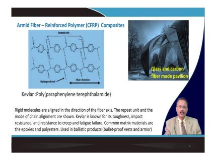
This aramid fiber which is having a technical term Kevlar which is poly paraphenylene terephthalamide; so, that is the technical name of this fibers. So, they are basically rigid molecules along with the fiber length; along with this direction and then they are bonded by hydrogen bonding they are very strong.
