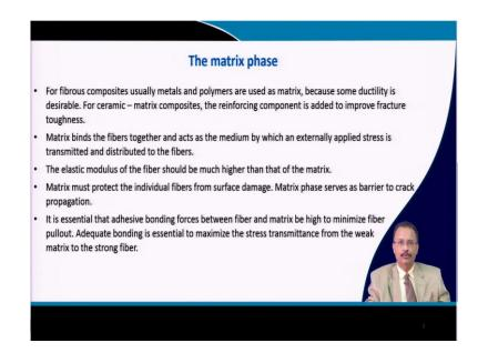
So, depending on this kind of fabrication protocol you will have; the mechanical property will be grossly affected. Now, in the matrix phase if you consider for fibrous composite; usually metal and polymers are used because of the simple reason that metal and polymer, they exhibit some kind of ductility.
