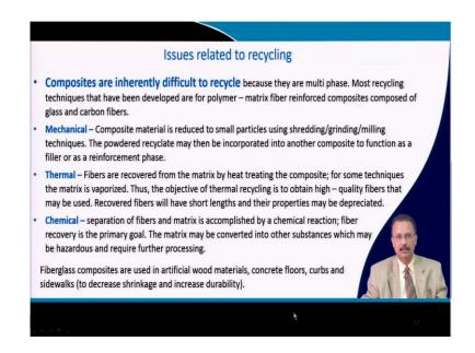
Now, with respect to the thermo plastic material; it is difficult to recycle the composite because they are having multi-phase material; fiber is there, resin is there. So, most recycling techniques that have been developed are for the polymer matrix fiber composite; whatever has been developed so far; that is to get out the fiber because the fiber material is relatively expensive.
