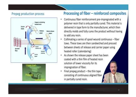
Second one is we called a prepeg production process and here this is a pre coated fiber; as you can see. So, pre coated fiber it is lightly cured and then it is sold, so whoever is using it; they have a resin impregnated fiber piece already and then they do the final processing and followed by curing etcetera. So, it is also a continuous fiber reinforce; pre ignited with a polymer resin that is only partially cured.
