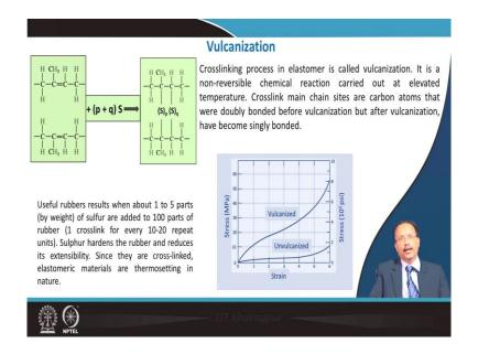
So, the process of vulcanization is nothing but cross linking of this elastomer as you can see that; you take the rubber molecule and then you react it with sulfur. So, the crosslink main chain sites are carbon atoms were doubly bonded before vulcanization and after vulcanization, it is singly bonded.
