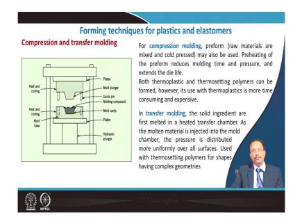
Now, for compression molding, I mean you can use both of them as you can see it is just a some type of press where you can simultaneously heat this also. So, the preform in the form of a either a mix or a cold pressed pellet, that is used. So, first you need to preheat it, so that reduce the molding time and then you just press it from the shape and then keep it hot and then cool it down and take it up.
