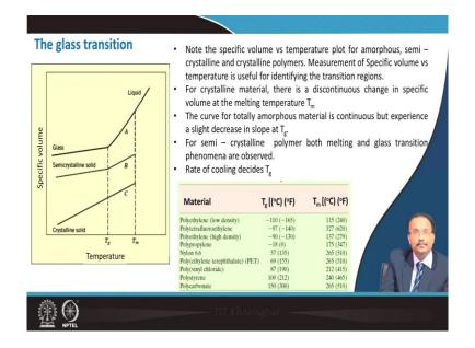
So, if you consider the specific volume versus temperature plot of a amorphous polymer and a semi crystalline polymer which is much different than the crystalline solid. So, specific volume is nothing, but the reciprocal of density right the v by m is the reciprocal of the density. So, in case of a purely crystalline material you see that there is a specific melting temperature and the specific volume is dramatically reduced here and the slope is reduced at the solid state.
