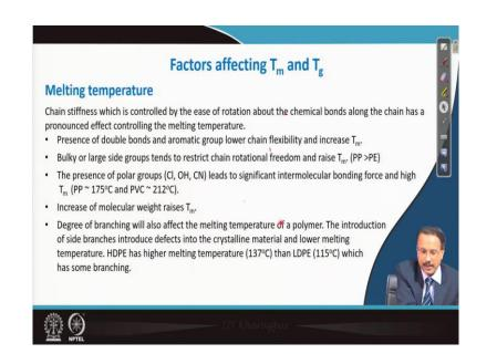
Now, the melting temperature this is affected by the chain polymer chain stiffness, which basically is controlled by the easiness of rotation about the chemical bonds along with the chain has a pronounced effect to control the melting temperature.
