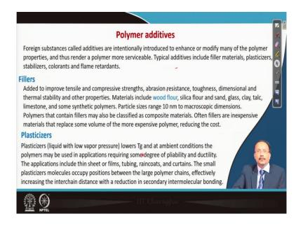
So, these two are the main mechanism of polymerization additionally, you may would like to add foreign substances we call its additive is intentionally introduced in the polymer to make it more serviceable. So, these are called filler materials or sometimes plasticizers are used, sometimes coloring agents are also used and sometimes fire retardant materials are used.
