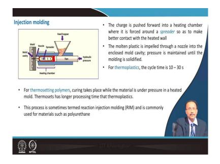
Injection molding is also used in case of thermoplastic polymer as well as thermosetting polymers in case of; thermo plastic polymer the cycling time is quite less. So, the charge as you can see is pushed here there is a ram and is a hot zone here. So, you first push it. So, it the pressure is pushed here and the polymer goes to the mold unless it is solidified.
