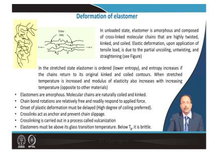
So, you can see that; the during the deformation in the unload state, the elastomer is amorphous and composes the cross-linked structure molecular chain they are highly twisted, somewhere it is kinked, coil formation is there. So, elastic deformation upon application of the tensile load is basically, due to partial uncoiling that you can see it is straighten up. So, some kind of uncoiling is taking place and twisting also is taking place and it is straightening so, it straighten up.
