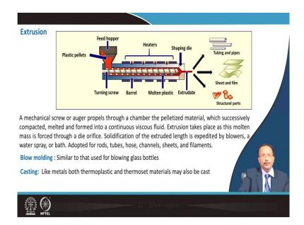
Extrusion is another technique a mechanical screw is here that propels through the chamber and where pelletized material is used initially, from the polymer it is pelletized and they form a viscous fluid extrusion takes place in the molten mass here is pushed through a die orifice.
