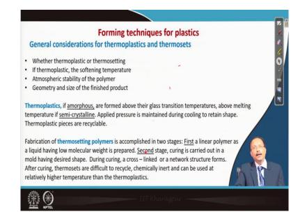
After that there comes the forming techniques of the plastic. So, the in general consideration whether it is thermoplastic or thermosetting, this if it is thermoplastic, then what is the softening temperature, what is the atmospheric stability of this polymer and also whether it is a simplified shape that you are trying to make or it is a complicated shape.
