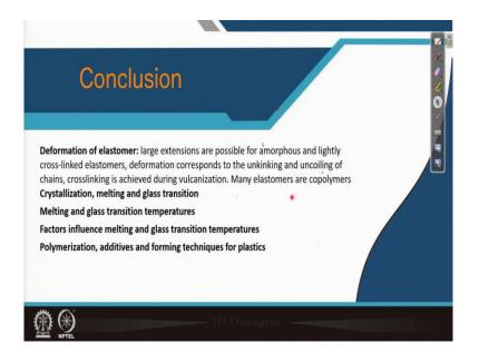
So, in this particular lecture, we talked about the deformation of the elastomer: and large extension is possible for amorphous and lightly cross-linked elastomer and deformation corresponds to the un kinking or uncoiling of the cross chains, crosslinking is basically achieved during vulcanization. Many elastomers and called copolymers are considered for this purpose.
