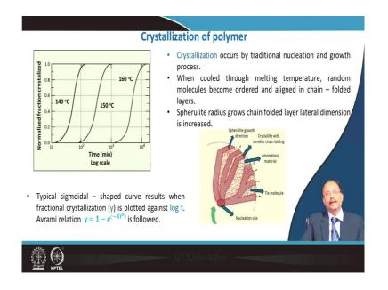
So, crystallization of the polymer actually occurs from its molten state by nucleation and growth process. So, when it is cooled through the melting temperature this random molecules they are ordered and in the chain-folded layers.
