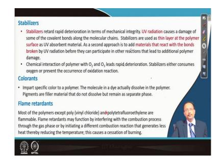
Stabilizer they are basically used certain polymers they deteriorates when you have UV radiation or when it is exposed to oxygen ambient. So, this stabilizer these are used in the polymer that either absorbs the UV radiation or either consume the oxygen's to prevent this kind of deterioration of the polymer.
