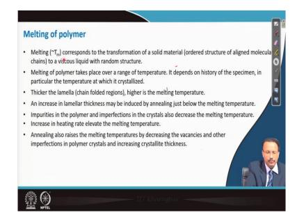
Now, the melting corresponds to the transformation of a solid material of ordered structure of aligned molecules chained to a viscous liquid with random structure. So, during melting it takes place and usually it is having a range of temperature not a specific melting point. And, that depends on the history of the polymer especially the temperature at which it was crystallized. Usually, thicker the lamellar the chain I showed that the folded regions higher is the melting temperature.
