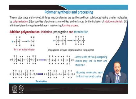
So, polymer are synthesized and processed there are three distinct kind of steps. The first one is of course, polymerization which briefly I introduced in my first lecture; and the properties of the polymers are modified by inclusion of different types of additive material and once you are ready with the polymer, then the desired shape is given by various types of forming process.
