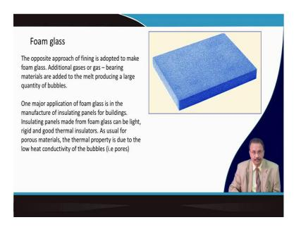
Foam glass is important where it is opposite to the bubbling effect because, as I told that bubbling is not good, but for some purpose we need bubble in the glass. So, the transparency is lost because lot of air bubble is there inside the glass and due to that lot of light scattering will take place so, it is no longer a transparent material, but it is a highly porous material and it is light weight.
