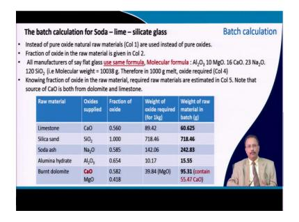
So, as I have said that instead of pure oxide natural materials that is used to make it actually commercially economic. So, limestone is used silica sand is used that is given in column number 1. Now, fraction of the oxide in the raw material is given in the column number actually it is column number 2.
