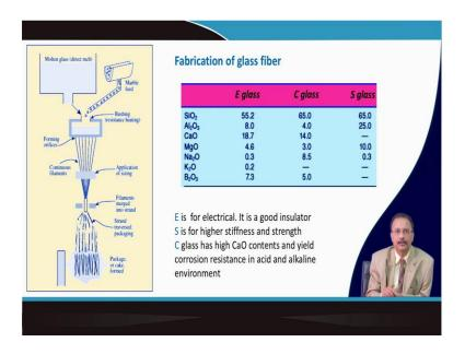
Finally you know about the glass fibers, which we have used for the reinforcement and this is in short that how the glass fibers are made. There are various compositions of these fibers and we call its E glass that is for the electronic purpose where it is having a good insulator. So, you take the glass melt or you can use the glass marble here in the molten form; and then there is a turret here.
