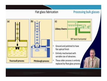
So, it has a different process name the Foucault process or Pittsburgh process depending on the place where exactly it was generated and these are all vertical process of drawing, but this Libbey-Owens process here the glass is 90 degree bent here right. So, this is 90 degree bent and then you form a flat glass bents. So, since either it is going through roller or most of the cases it is going through roller as you can see.
