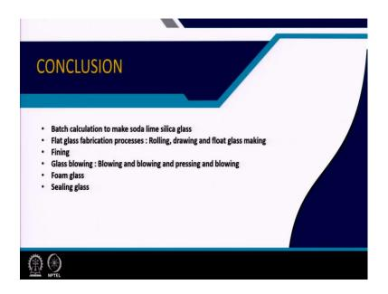
So, in this particular lecture we talked about the batch calculation to make soda lime silica glass, flat glass fabrication process including rolling and drawing which are obsolete nowadays almost it has taken over by the float glass making process. The concept of fining sometimes it is required sometimes it is not required.
