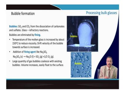
So, once the glass is coming out from the so called forehearth then it is something like this and the major problem comes that it contains bubble, and the bubble is coming from sulphur dioxide and carbon dioxide form the dissociation of carbonate which you have used you have used in the raw material and also the glass tank furnace refractory and the glass melt they are interacting and it forms bubble.
