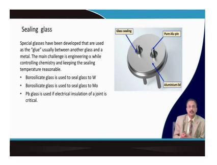
Another one is a sealing glass this is very important because in certain electronic application you need to insulate this two conductor so; there is a glass seal here in between. So, this inner material is glass seal and this is aluminium pin and this is also metal body. So, special glass have been developed for this kind of sealing that used basically as a "glue" between another glass or glass metal.
