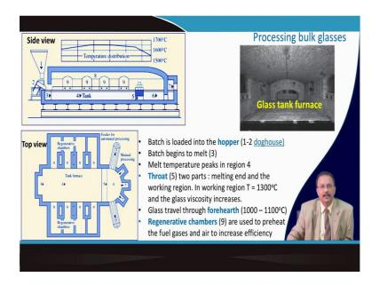
And this kind of calculation this is usually done in undergraduate level ceramic engineering course and this is industrial stoichiometry a typical subject name that is given for this kind of batch calculation. Now, once you calculate the batch actually this is a side view of a sorry elevated elevation of a glass tank furnace and this is the actual glass tank furnace for processing of the gas.
