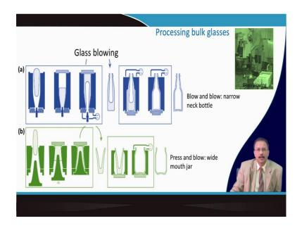
So, glass blowing is another so that is all about the flat glass process, otherwise you can use glass blowing and here in case of glass blowing you used gob this is called glass gob. And first due to gravity it falls here and then you apply a air pressure and the mould is something like this. And then you get a glass article out of the mould and again you blow inside a mould. So, this is blow and blow process to get a narrow neck bottle like this.
