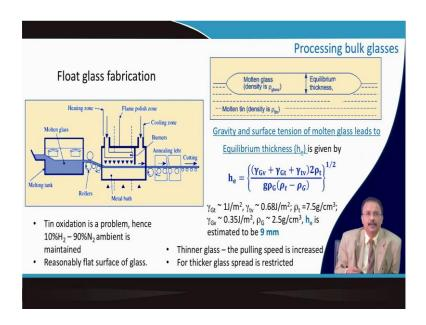
And in case of float glass the glass is coming from this region and then it is the lay the roller usually this is similar kind of thing, but then it is spread on molten glass sorry molten tin. So, molten tin it is floating here and once it you spread this one, you see that it has its own gravity gravitational force and also the surface tension right.
