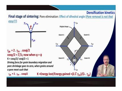
Now, in the final stage of sintering what is eventually happening is the pore is getting shrink right. And, it depends on the grain boundary also grain boundary initially, there were carved grain boundary which is becoming flatter and flatter. So, it turns out to be flat.
