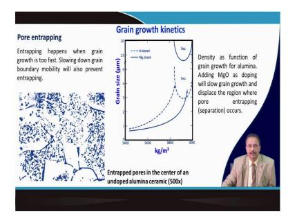
So, this is one example of the pore entrapping inside the grain. So, entrapping usually happens when the grain growth is too fast. So, when the grain mobility is too fast, then it will acquire the pores very fast within the grain structure while the grain growth takes place. And slowing down the grain boundaries of utmost importance, otherwise it will have a almost a very porous entrapped microstructure.
