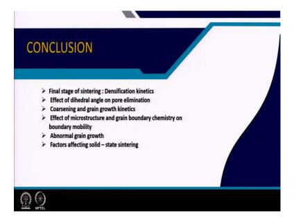
So, in this lecture final stage of sintering particularly densification kinetics, they are described effect of dihedral angle on pore elimination, that has been illustrated coarsening and grain growth kinetics have been introduced, effect of microstructure and
