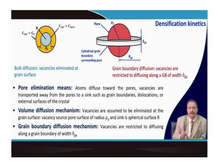
So, we actually described that what happens during bulk diffusion. So, vacancies they are eliminated at the grain surface. So, the pore elimination I meant that atom diffuses towards the pore vacancies are transported away from the pores right. So, it is a counter current kind of situation.
