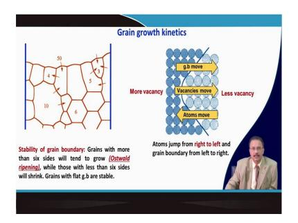
So, the stability of the grain boundary is important and grains with more than six sides will tend to grow. Because, already we were discussing about it, and this is sometimes called Oswald ripening and whatever is less than 3, they will shrink. And this can be understandable from the concept of the curve surface. So, here you can see that in this area, it will have more vacancy, because this is concave in nature and this will have less vacancy.
