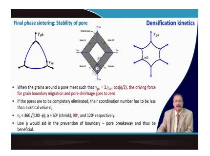
So, this is a stable structure and this structure is unstable, because if it is less than the numbers, here it is 4 it is less than this then it will try to shrink. And if it is more than this then it has lot of energy to grow. So, when the grains around the pore meet such that this relation is valid. The driving force for the grain boundary migration and pore shrinkage goes to 0. If the pores are to be completely eliminated, then the coordination number has to be less than the critical value.
