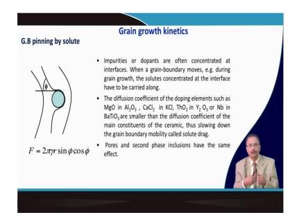
Now, if the grain boundary movement is related to the grain growth. And, if you want to stop it then the grain growth kinetics is grossly stopped by grain boundary pinning. So, you can put impurity atoms inside the material, they are often concentrated at the interface when the grain boundary moves during grain growth.
