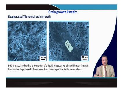
So, this is the example of a exaggerated grain growth. So, this exaggerated grain growth is associated with the formation of sometimes a liquid phase or a very liquid film at the grain boundaries and liquid results from maybe the dopant or from some impurity. And grain boundary mobility is very much enhanced and some of the grain, they are of abnormal size range that you can think of.
