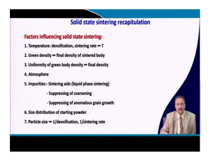
So, finally in solid state sintering factors that influence the solid state sintering is temperature, that densification and sintering rate that is proportional to the temperature that we are using. Green density is important that is proportional to the final density of the centered body. Uniformity of the green body density that is proportional to the final density.
