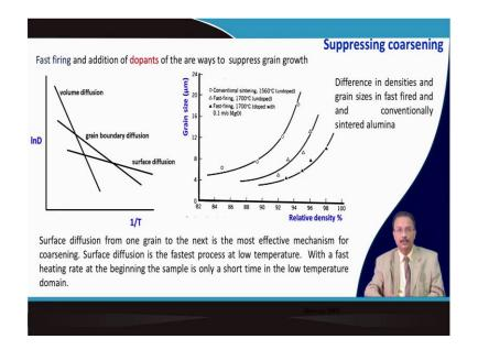
So, fast firing is one way that suppresses the grain growth. Now, we are talking about the grain growth. So, as you can see that if I plot this density coefficient the coefficient D as a function of temperature, that at relatively lower temperature the surface diffusion is operative.
