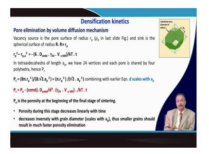
Now, the pores need to be eliminated at the final stage of sintering that is by diffusion process, and already I introduced this figure. This is the actual grain which has formed from the particle at initial stage. And through the grain boundary you can see all the pores are eliminated and only at the junction point among the grain you have the porosity left. So, vacancy source is the pore surface of radius r p, I am assuming now although in the figure it is showing rho p, but it is shown r p.
