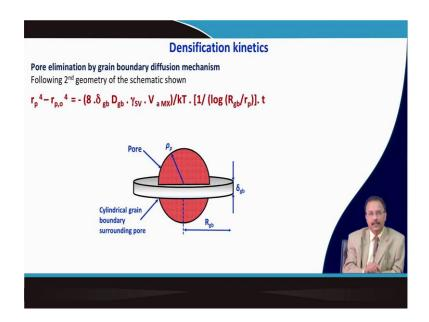
Pore elimination when it takes place through grain boundary diffusion mechanism, following the 2nd geometry which I have shown that this one. One can write this relation between the radius of the pore and initial and final stage. And this is valid relation for the pore elimination for this kind of geometry.
