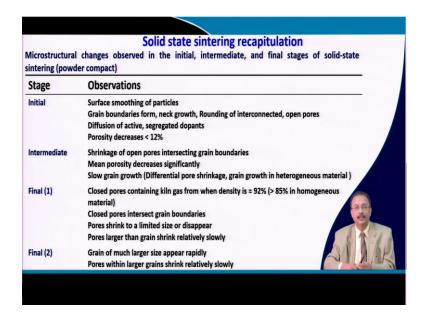
So, now I will just tabulate or summarize that different stages of sintering, because I have been talking about sintering for quite long duration. So, let us see what are the important point as far as the microstructural change occurring in these three phase of sintering solid state sintering.
