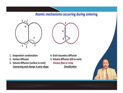
Now, just look at the different atomic mechanism that is occurring during sintering. So, as you can see that these are your initial 2 particle and these two particles they have come into close contact. So, it is forming a region interfacial region which will
