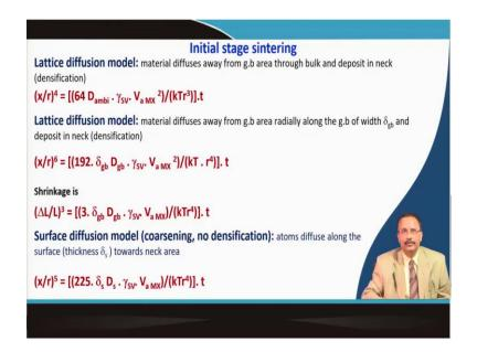
So, that is part of the initial stage sintering. Now if you do similar kind of calculation for other models like Lattice diffusion model. Then you will come up with all different types of relation and what you will have to see that how this x by r varies with the time as well as the particle size because this is miserable quantity right, time is measurable that is a sintering time and the initial particle size you know.
