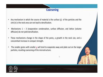
So, first let us concentrate the coarsening mechanism number 1, then 2 and then 3 these 3 will lead you to the coarsening. So, any mechanism in which the source of the material is surface of the particle and the sink is the neck area that will not lead to any kind of densification.
