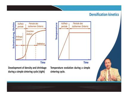
Now, the stage of sintering pardon for the language it is taken from a German slide. So, still the German things are there. So, initial stage it is here and then it intermediate stage this increases. The density and it is the final stage the it is almost asymptotic about 96, 97 percent. And corresponding heat treatment schedule is given here.
