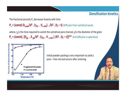
So, the fractional porosity decreases linearly with time. So, I can write the equation of fractional pore is related with the diffusion is involved and actually the a is scaled down with the d diameter of the so called particles and this is the diffusion from the cylindrical force which was that curved arrow. So, those kind of situation the fractional porosity reduction is given by this relation.
