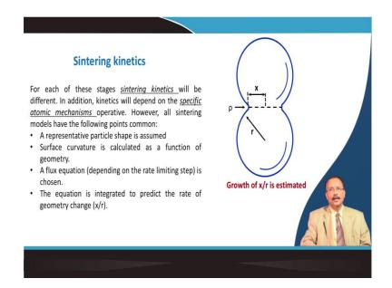
So, now we will talk about the kinetics of the sintering. So, for each of these stages of sintering the kinetics will be different. Kinetics will depend on the specific atomic mechanism operative. However, all this mechanism whatever I have just described they have something common in them.
