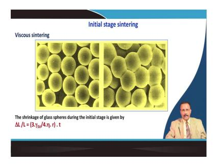
In case of viscous sintering this sprinkle law that is valid. So, shrinkage is given by this relation where as you can see it is a function of the viscosity of this glass sphere. Its radius as well as the time of sintering.
