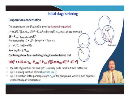
So, first let us consider the evaporation condensation mechanism. So, first I will ah choose a rate equation evaporate rate equation and usually the Langmuir equation is adopted. So, where the flux is j, which is equated with the evaporation coefficient which is alpha, del P is the pressure difference and m MX is the mass of the gas molecule because as I said it is going from the surface to the gaseous region and then it is deposited in the neck.
