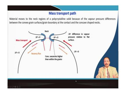
So, this was the slide from the last lecture where I was describing the mass transport path. Materials move from the neck region of a polycrystalline solid because of the vapour pressure difference between the convex grain surface and grain boundary at the contact and the concave shaped necks. So, that is already illustrated.
