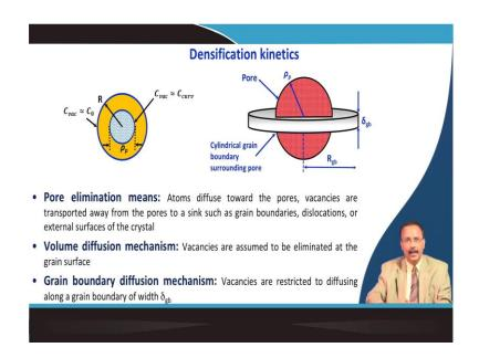
So, here you have a situation something like this. So, you have a porous region and then you have the granular region right. So, here it is your grain boundary this grains and it has this pores region in between right. So, the pore elimination means attempt diffuses towards the pore so covered the pore region. Vacancy is a transported away from the pore to a sink such as grain boundary dislocation or external surface of the crystal and then the pores are eliminated.
