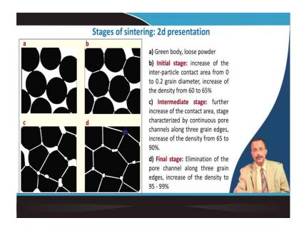
So, if you do it 2d presentation of the same phenomena which is which I just described. So, this is a green body is a loose powder in initial stage, inter particular contacts area is increases from 0 to 20 percent grain diameter, increases the density about 60 to 65 percent.
