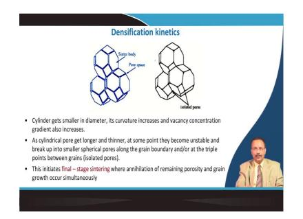
So, the situation is something like that the cylindrical cylinder gets smaller in diameter, here. So, as compared to this it is getting smaller here its curvature increases and vacancy concentration gradient also increases. Cylindrical pores get longer and thinner, at some point they become unstable and break up to smaller spherical pores along with the grain boundary or specifically at the triple point between the grains.
