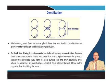
So, mechanisms apart from the viscous or plastic flow, that can lead to the densification or the grain boundary diffusion and bulk or volume diffusion. So, viscous flow is also that gives you sintering the shrinkage, but here you can see that in case of this grain boundary diffusion and bulk diffusion there is a notable shrinkage of the particle that is taking place.
