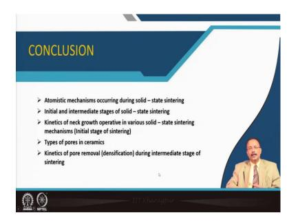
So, in this lecture I have introduced the atomistic mechanisms occurring during sintering the solid-state sintering process. Initial and intermediate stages of solid sintering I have explained. Kinetics of the neck growth operative in various solid-state sintering mechanism that is the initial stage of sintering that has been described the how x r varies with t and the radius of the particle.
