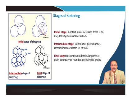
So, there are 3 prominent stage of sintering. The initial stage you see that the particles are something like this then they are coming into contact and in initial stage the contact area increases from 0 to about 20 percent and the density is also increased 60 to 65 percent so, that we call initial stage of sintering. In case of intermediate sintering you see that this curvature is gone.
