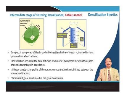
So, now we will talk about the intermediate stage of sintering and initial stage of sintering is over then it is more about densification and we will talk about the densification kinetics. In case of the initial stage of sintering we were worried about the neck growth x by r. So, kinetics was related to x by r.
