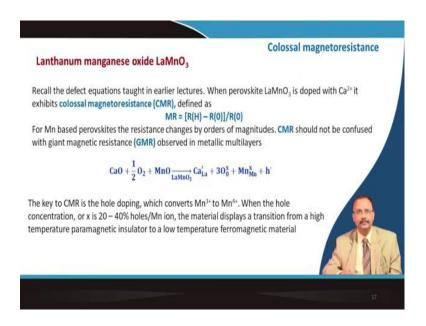
Lanthanum manganese oxide it is perovskite structure, this is also important material. And you remember that we talked about that you can change the defect state by aliovalent doping. So, once it is doped with calcium 2 plus, when you replace lanthanum with calcium 2 plus. Then, it exhibits a colossal magnetoresistance and that is defined as resistance with the field applied, it is much larger as compared to when there is no field applied.
