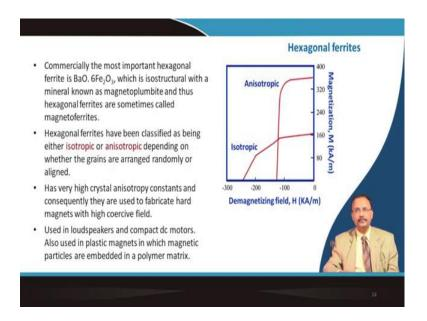
Hexagonal ferrite they are good materials for hard magnet and commercially the most important hexagonal ferrite is isostructural with magnetoplumbite, and this that is why they are called are magnetoferrites. And they have been classified either being isotropic or anisotropic in nature. So, when the grains are randomly oriented during the fabrication itself by putting a strong magnetic field you can align the grains.
