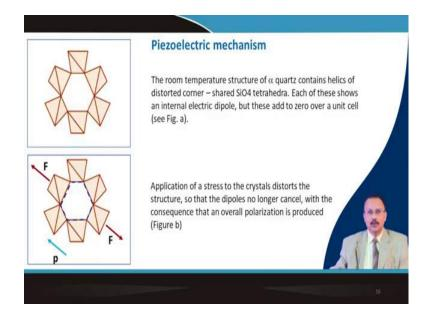
So, similar thing happens in quartz crystal. In quartz crystal, it forms a helix structure like this. So, here your Si ions are there in the oxygen tetrahedra. Once, you are applying a force then these lines of force are not matched. So, then it generates the so called piezoelectric effect in quartz crystal.
