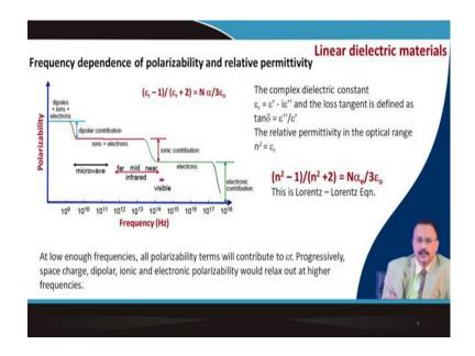
So, in an AC electric field, all this different polarized will source will not be actually contributing. So, at very high frequency, all this polarizability will relax out because they cannot actually follow the kind of the speed is not enough for ionic polarization or the dipolar polarization to follow it.
