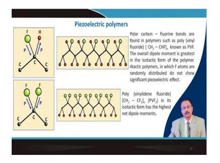
In certain polymer also this piezoelectricity is apparent and I have cited the example of polar carbon fluorine kind of bond which is having a intrinsic dipole. So, it depends that how this dipoles are oriented, whether you remember that we talked about isotactic kind of arrangement of the polymer.
