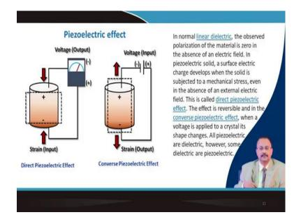
Now, we will talk about the piezoelectric effect. Mostly, there are two types of piezoelectric effect. In certain material when you are applying a stress, then you will see that it generates electricity. So, the polarization is related to the stress and not due to electric field.
