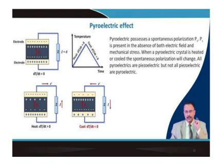
This type of material insulating material, sometimes it is also possible for you to change its polarization. Because what you are doing? You are changing the polarization that means the dipole moment per unit volume either by application of electric field. In case of linear dielectric, once you are applying the electric field, then the polarization is there. Once you take out the field, then the polarization is 0.
