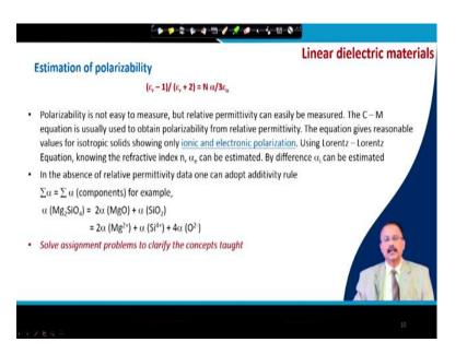
And now particularly, for ionic polarizability and electronic polarizability, you can separate it out the individual component. I will just hint you how to do that, but exact assignment problems are illustrated just to make you understand this concept. So, this is my equation of polarizability and that its relationship with dielectric permittivity.
