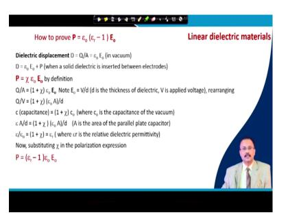
Now, as I told that this can be proved, this polarization and dielectric field, this linear relationship is given by this relation, it can be proved. So, we will introduce a term which is called dielectric displacement, which is nothing but the surface charge density. Q is the surface charge and area is involved here.
