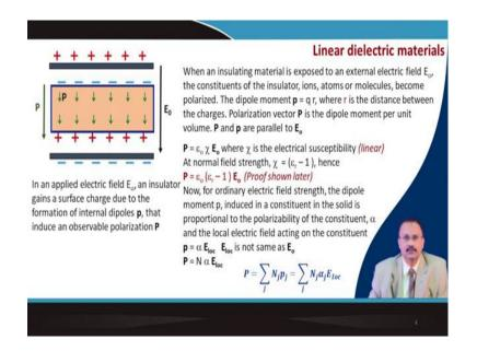
So, the situation what is happening can be explained by this figure. So, initially you have charge here and then, you have inserted a dielectric material. So, something is happening in this material, you can see that in the material itself, there are small dipole moment that is being created.
