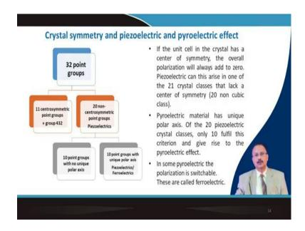
So, this set of material, this multi functionality is dependent on the point group on the symmetry. There is no scope for me to go into details about the details of the point group, but there are 11 centrosymmetric point group material and which are not piezoelectric in nature.
