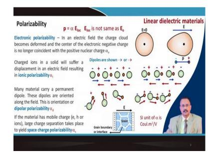
Now, as I said polarization could be of different types and remember, this basic relation that this dipole moment is related directly proportional to the field that is being applied to this different types of polarizability. The first type of polarizability is electronic polarizability, when you are applying a field in the positive direction.
