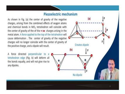
So, the piezoelectric mechanism can be understood by this fictitious tetrahedral material and as you can see that if I apply a stress here, then this cation which is sitting in the tetrahedral void, they will be shifted here. So, the electric lines of force of this orange atom will not coincide with the electric lines of force of this positive cation.
