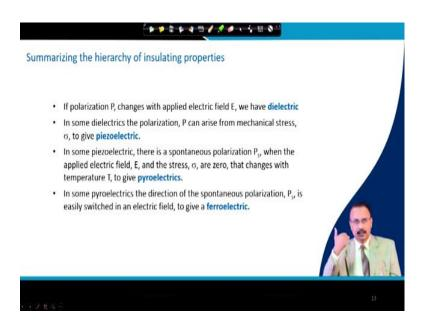
So, polarization as I said that certain material could be dielectric material, certain material can be piezoelectric in nature when polarization is changed by stress, some material can be pyroelectric in nature, where the polarization can be changed by the application of temperature change and in certain material, this polarization value is switchable.
