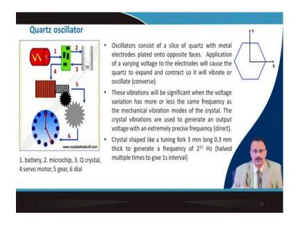
And this quartz is a time keeper. You know that the quartz crystal is used to make the watch and this is due to the fact if you take a single crystalline quartz and you can have various types of cut; X cut, Y cut or XY cut. This is possible and what is happening that this quartz crystal, it is in the form of a tuning fork.
