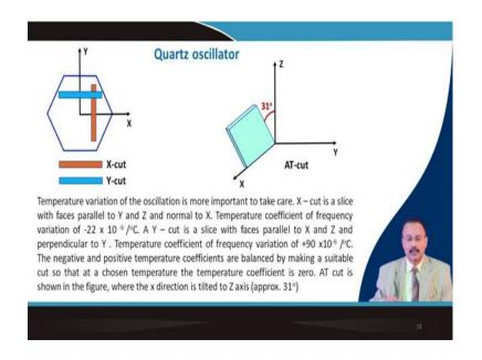
Now, as I said that this kind of cut is very important because you will have to take care of the thermal expansion coefficient. Thermal expansion coefficient should not change with the temperature. So, therefore, this special cut, we call it is a AT-cut, where this X axis is slightly tilted to the Y axis.
