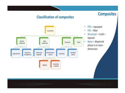
To give you the brief overview of the classification, which already I have described part of my earlier lectures. We have already talked about particle reinforced composite; where both large particle reinforcement and dispersion strengthened reinforcements were covered.
