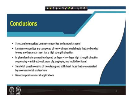
So, in this lecture we talked about structural composite laminar and sandwich type. Laminar composite composed of two dimensional sheets, they are bonded to one another in the high strength direction. And, sandwich panel consists of a strong stiff sheet faces that are separated by a core, which are softer in nature. And, finally, we talked about nano composite and their perspective applications.
