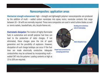
Mechanical strength enhancement takes place with a light weight polymer nano composite that is basically again use carbon nanotube into epoxy resin. And, here we use about 20 to 30 weight percent are normally required to make this kind of nano composite. And, wind terminal sorry wind turbine blade for generation of the electricity or also tennis racket, you know or baseball bat they are used out of this composite.
