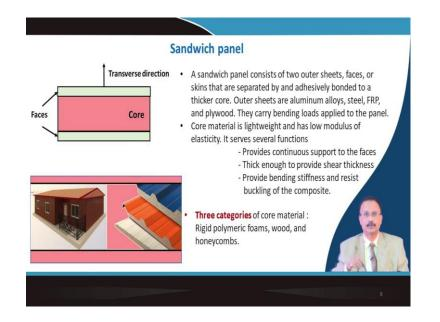
The second types of structural composite is sandwich panel type. And, you can see that, basically it is having a core, which is having a thicker structure. And, on top of this core you have a relatively stiffer, outer sheets at the face. So, actually this face strong material they are separated by this core material, which are relatively softer. So, this outer sheets they are usually aluminum alloy steel can be used, fiber reinforced plastic can be used, plywood can be used.
