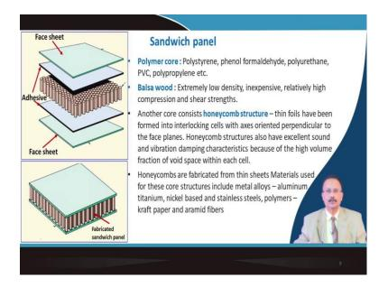
So, this is the actual structure of this kind of sandwich panel. As you can see the first one is the face sheet, the first part. The second one is the adhesive layer and then you have this core layer. Here typical core is of honeycomb structure; then again you have another adhesive layer and finally, the face layer. So, all of this are laminated they are pressed to form this kind of light weight, but strong composites.
