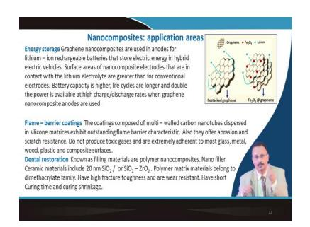
Another thing which is coming up quite extensively is in the area of energy storage. You know the graphene is being used or reduced graphene oxide, which is having reasonably good electronic conductivity. They are used with the anode material, I have cited one example, which is ferrosoferric oxide Fe 3 O 4 and this is embedded in a graphene sheet.
