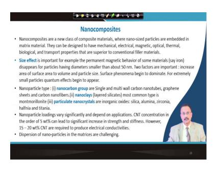
Now, the final thing that, I would like to address is the nano composite. So, nano composite as you understand this is a new class of material, where the reinforcing agent it is in nano size. Dimension nano is a bit blurred, but whatever below 100 nanometer
