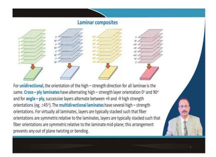
So, if you see the configuration of this laminate structure, you can see the first one this is unidirectional. So, all the fibers of course, they are having much higher tensile strength as compared to the matrix. So, they are all oriented in one particular direction. So, therefore, these are 0 degree, we have mentioned it.
