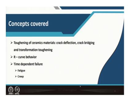
In the last lecture, we introduced the concept of toughening of the ceramics and the concept of fracture toughness which was related to the storage of elastic energy upon certain application of tensile stress into the ceramic. And then, at a particular critical length of the crack, this crack will start to propagate and it will have two surfaces and the crack, the elastic store energy is released.
