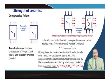
In designing of ceramics we will discuss that having that small fracture toughness how we can manage the situation. Now the strength of the ceramics usually they are very strong in compression because as you know in case of tension your crack if it is favourably oriented like this it will start to propagate right. Because as I told that tensile force it propagates to the this direction.
