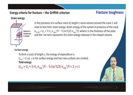
Now, we are talking about the strain energy continuing now you imagine that in that case you introduce a small crack at the surface. So, the presence of the surface crack the length I have assumed it is C and it has some kind of volume around it and it will start to propagate because at one point it cannot withstand that energy. So, the strain energy this part will be there and then depending on the shaded area this volume this will start to release this energy will start to release right.
