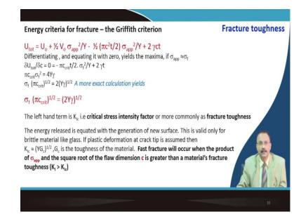
So, the crack dynamics inside the material is also very important to give you a good fracture stress. So, we can have this maxima by differentiating this equation and equating this total energy with the crack length with 0 with standard mathematics and you come up with this relation.
