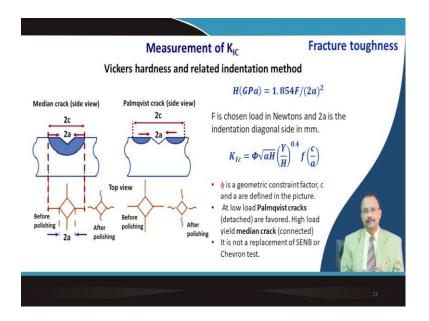
Another way to measure the fracture toughness is through hardness measurement. Already I introduced the hardness part and we talked about the micro hardness. So, hardness is given by these dimensions this 2 a this dimension is given the anvil dimension and this dimension is 2 c.
