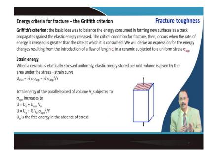
So, theoretical strength whatever you can get from the calculation like Y by 12 or Y by 15 in practical case you your fracture stress is much much lower than that and this is due to the reason of having crack and void inside the sample. So, when I will talk about the sintering you will see why sintering is so, important for ceramic material in particular
