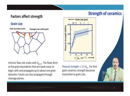
The strength is affected by grain size because of the fact as you can see that in one grain this crack length is defined and actually the crack propagates by this grain boundary. So, you have a relation I have shown you that applied stress is multiplied with your crack length to the power root. So, now, it scales with the grain size.
