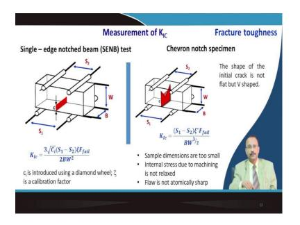
Now, how this fracture toughness you exactly measure? It is measured by a 4-point bending test I already talked about 3 point bending. So, it is something similar to this now this material is well polished this beam and then a small notch of c length.
