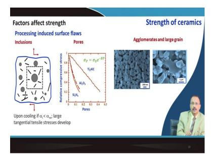
So, processing is important any kind of inclusion if they have different thermal expansion coefficient then there will be micro crack formation which is not good for your material. So, if the pores are there then of course, the strength will be reduced and if there are agglomerates in the material to start with or there is exaggerated grain growth during sintering then the strength will get reduced. This factor I will elaborately discuss when I will talk sintering aspect of ceramic material.
