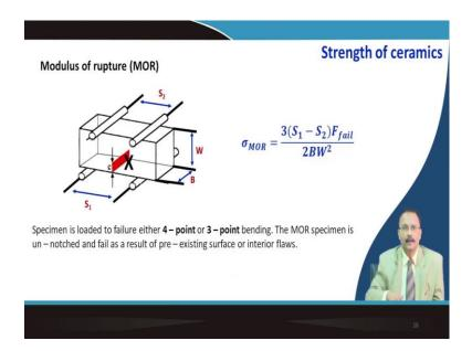
Modulus of rupture is another thing that also I mentioned in my last lecture that it is again 4-point bending test, but now unlike the fracture toughness test you do not have this small crack here. So, modulus of rupture is actually estimated from this relation according to the ASTM specimen and this will give you a fairly good idea of a mixed type of strength that this material that you have.
