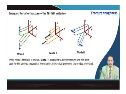
Now, actually we are interested in this type of mode where the crack propagates in perpendicular to the applied stress. Apart from that you have mode two also possible where you are applying a shear stress and the crack is propagating in parallel to this or you can have a shear stress something like that we call it is a tearing kind of force and the crack propagates in this direction.
