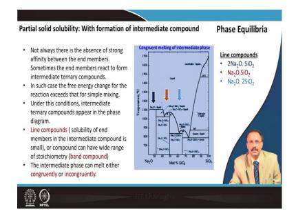
Now, let me describe a case where partial solid solubility with the formation of an intermediate compound takes place. So, now, it is not a perfect solid solubility some kind of intermediate compound is also forming. So, this is a typical diagram of sodium oxide and silicon dioxide. When I will take the glass part I will explain it in details. So, this is a typical phase diagram. And there is a little bit affinity between these two, so the phase will form.
