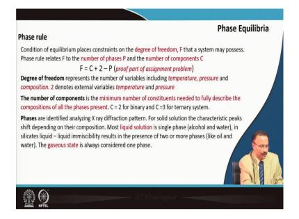
So, let us first introduce the phase rule and this phase rule as you can see in the relevant equation is related to the degree of freedom. Degree of freedom is denoted by F. Component of the system, if it is a single component system or multi component system three components system, so that is a part, and these 2 determines signifies the temperature and pressure, and P is the number of phase.
