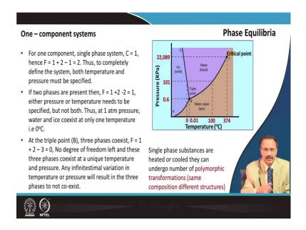
So, in single component system, component is 1, degree of freedom will be 1 plus 2 minus phase is 1. So, if the degree of freedom is 2, then the complete if you want to define a single phase system, then you will have to specify the temperature as well as pressure. When two phases are present, then your degree of freedom you put it in that equation degree of freedom is 1, so either temperature or pressure you will have to define.
