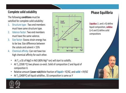
Now, in the complete range of solid solubility, there are certain rule it must be followed. If two component – two ceramic component forming a solid solution, then there should be structural compatibility. So, in this case nickel oxide and magnesium oxide both are FCC type. The constituent cation because anion is same.
