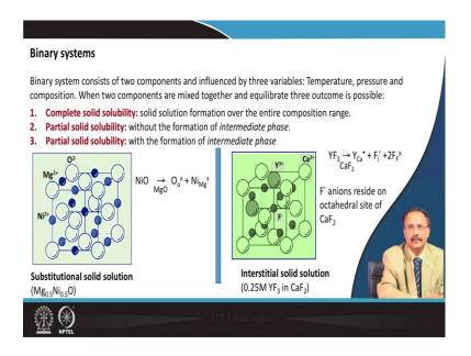
So, the polymorphic phase transformation, I will take part of the course for a single component system in the phase transformation lecture. So, single phase system in ceramic, it is important for barium-titanate, for silicon dioxide. So, we will be taking that details of the single component single phase diagram. So, for the binary system, you have three different possibility. One is a complete range of solid solubility. I talked about the defect.
