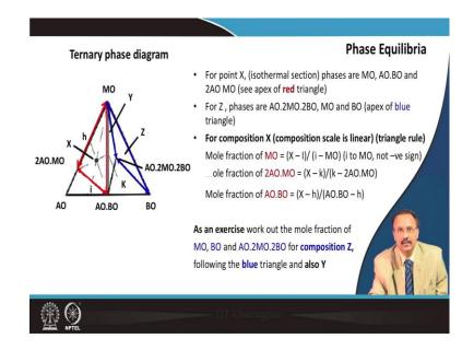
Now, in ternary phase diagram, again for a eutectic reaction, you can identify the mole fraction of this constituent phase. So, in that case, you will have to draw a triangle. For example, if you want to know the composition of X, then this X is basically within this particular triangle which I have marked rate. So, this is also an isothermal section and it constitute phase which is MO, then AO, BO, and 2 AO and MO. So, it is lying in between this.
