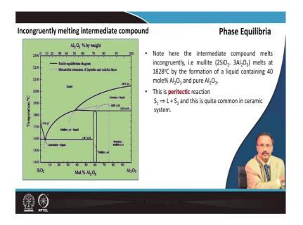
But here it is also a bent diagram as you can see. But when it melts then the composition is no longer similar, so for example, this mullite, I am talking about when it melts then the composition is somewhere here, somewhere here, this composition you can see which is very different. So, this reaction, this temperature, whatever reaction is taking place this is known as peritectic reaction.
