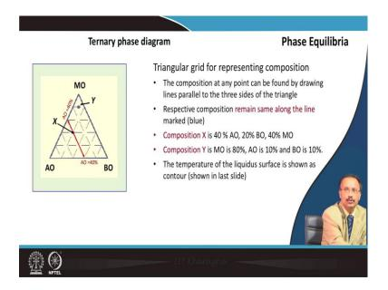
Now, we will learn how to read this ternary phase diagram. So, in order to read the composition of a system in ternary phase diagram, you will have to draw this equilateral triangle. And at any point say X, this composition if you are interested to know, so you will have to draw parallel lines here. So, one parallel line correspond to this particular line.
