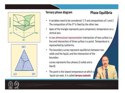
Now, we will talk about the ternary phase diagram, where there are three component which is present. So, you have three component present, and temperature, and pressure. So, totally there are five variables. If you consider the pressure remain constant, then there are four variable system.
