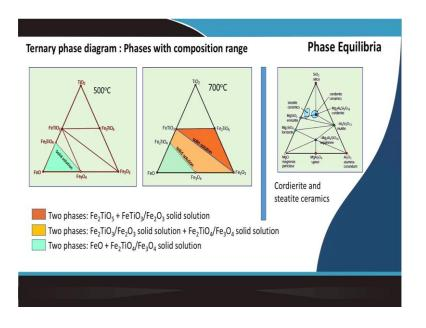
Sometimes, it also follows a solid solution not always it is a single compound. So, it also forms a solid solution. So, one example I have cited in this system titanium oxide, iron oxide and Fe 2 O 3. So, these three compositions if you take, the intermediate composition several phases forms – this Fe 2, Ti O 5, Fe Ti O 3.
