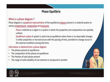
Now, the phase diagram is basically a graphical representation of the equilibrium phase that is there in a particular material system. This equilibrium phase present in the system at different temperature, composition of the material as well as in different ambient pressure. So, the phase that is defined as a region in the system in which the properties or the compositions are spatially uniform, so that is defined as a phase.
