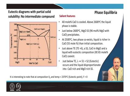
Then let us come to the next case which we call a eutectic diagram. And again I will try to explain the salient feature of this eutectic phase diagram. You start with a liquid which is having 40 percent of calcium oxide and start to cool it. So, as I said above 2600 degree Celsius, it is all liquid; liquid phase is stable. Just below 2600, magnesium oxide solid solution will form, and the composition will be about 96 percent of magnesium oxide. In calcium, little bit calcium will also be there.
