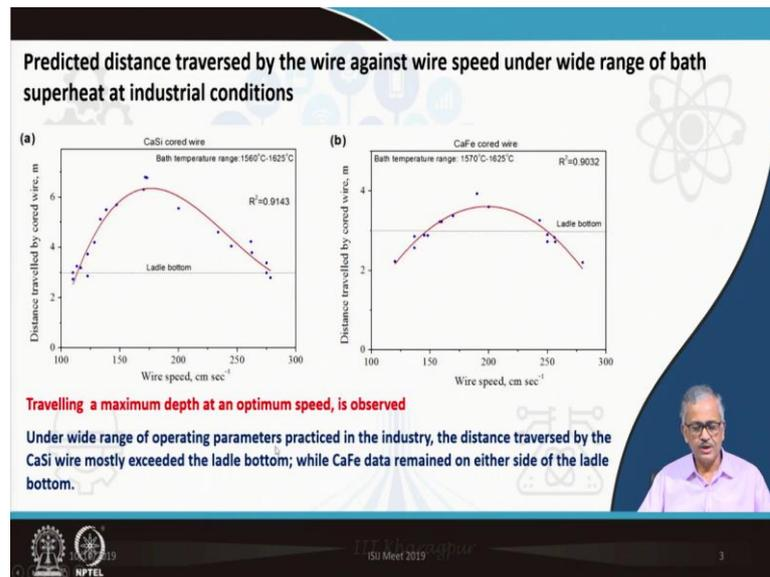
Here we have calculated the distance traversed by the wire in actual industrial melt against the range of values of wire speed (100 to 300 cm/sec) and bath superheat (1560 to 1625°C) under actual industrial operation.
