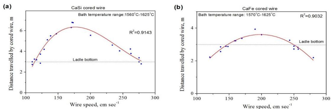
Figure 24.1: Mapping of predicted distance traversed by the wire in actual industrial liquid bath against widely varied wire speeds for a range of bath superheats under industrial operating conditions: (a) for calcium silicide (Ca-Si), (b) for Ca-Fe.
