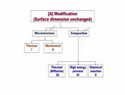
So, in terms of dimensional changes where surface dimension is not changed, but only we modify as I said, we can change only the microstructure or composition and these are the different methods.
