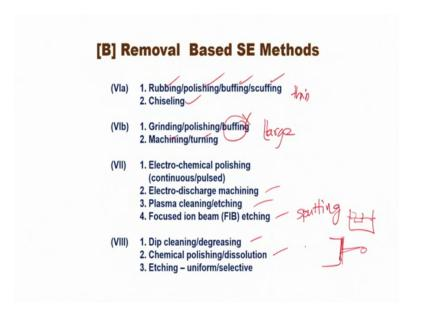
So, we can do anything like say rubbing, polishing, buffing, scuffing, chiseling heavier or when we deserve here that the amount of material removal is a thin or small and here the material removal is large. So, we can think of grinding, polishing or machining turning and so on, buffing is not quite correct because generally the material removal is very small here. We can also remove materials and clean the surface and make it truly
