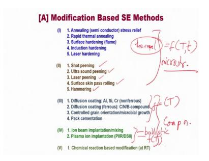
And if we go deeper then these are the techniques we have discussed in various times, anything starting from a needling, rapid thermal annealing, surface hardening, induction hardening, laser hardening or any other hardening process. So, it this is basically a thermal process, all these are essentially at thermally activated process. So, where we so,
