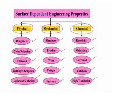
So, we as we just now mentioned we divided them into three major classes; physical, mechanical and chemical. For example, roughness, color and reflection, image emissivity or emission characteristics, wettability adsorption, adhesion cohesion all these properties we club them under the physical properties.
