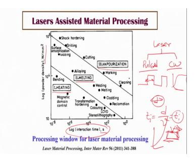
Surprisingly though the scope is very; very large, but it is fairly easy and you can as I said you can do three types of processing only heating within the solid state or melting, then solidification or vaporization condensation. So, these three caskets can all be controlled.
