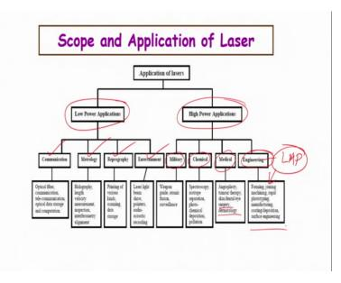
Now, the laser actually has multiple possibilities of application. So, there are two major scopes two major types of applications, typically in terms of the power. So, in case of low power applications we are talking about communications, metrology measurements, reprography, entertainment and various forms of them.
