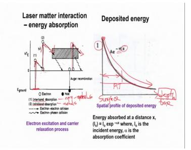
So, this is what I was mentioning a few minutes ago, that either you excite the electron from the from the valence band to the conduction band and then further excite to higher energy state or if it is a metal then you already have electrons in the conduction band. So, you excite them and then subsequently they get de excited.
