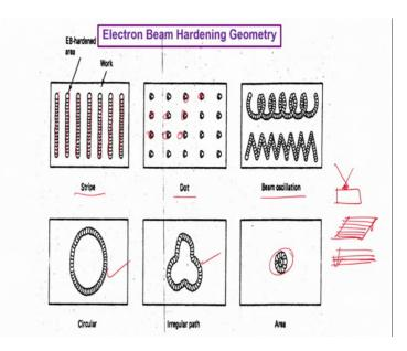
The various geometries are possible, you actually can make stripes or make dots or circular dots or you can create oscillation of the beams and create certain complicated shapes. So, the point is that on a flat surface for whatever reasons if you would like to treat these kind of stripes or create these kind of stripes and leave the portion in between unaffected or you create certain patterns like this, which are may be circular or some geometric shapes.
