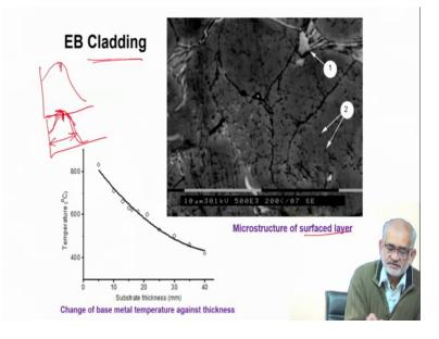
So, this is a typical microstructure done on a tool steel. The temperature that the metal seize will decrease from the surface to the core and yesterday we did discuss about the way the ion beam interacts with metal. And there if you recall while discussing ion beam we did not say that the deposition profile is Gaussian and the peak is below the surface. The same deposition profile or the feature applies to electron beam as well.
