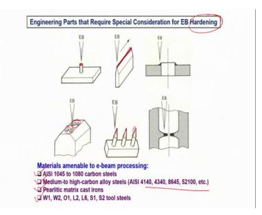
So, we can have; we can for example build components like this vertically, we can build a component like this or we can irradiate only this part only this part and not elsewhere. Similarly, we can irradiate or heat up only this part or build a material at this sharp part of the shear blade and not the rest of it.
