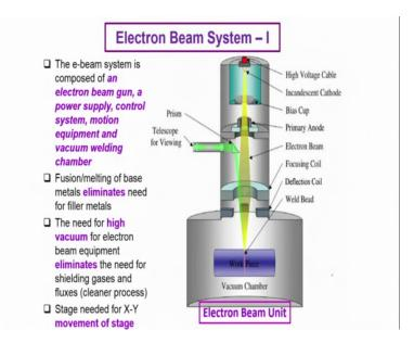
So, let us go straight away into the configuration you have seen this view graph in the previous lecture. So, essentially we have these are the constructional features we have an electron beam gun, we have a power supply which applies very high negative potential difference to give you a kinetic energy to the electrons, we need a control system, we need an sample manipulation stage and of course, very high vacuum chamber.
