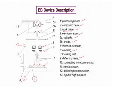
So, this is the processing zone the so called processing room, you also need a compound desk on which the substrate which may be a small light one or may be a very large thick one and you also need to be clamped well. So, that it does not deflect during their processing period.
