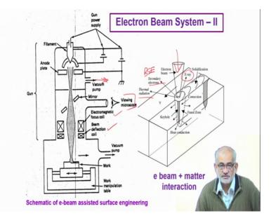
So, this is the overall setup this again is repeated from the previous lecture just to bring home the point that the same configuration and we require the similar mechanisms for focusing for deflection, also we need a viewing port and we need to maintain very high vacuum before we start the electron flow. And eventually, once the erudition occurs then this is how the surface of the solid gets I mean undergoes melting process.
