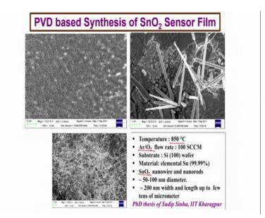
Actually, you can create special conditions of maintaining a specific temperature and mixture of argon and oxygen to create certain oxide layer. So, you actually heat up tin and introduce very low amount of oxygen and allow certain reaction to take place and this reaction can lead to formation of a very thin tin oxide layer. And this tin oxide layer the beauty of it is that actually by controlling the process parameters you can change the aspect ratio very significantly.
