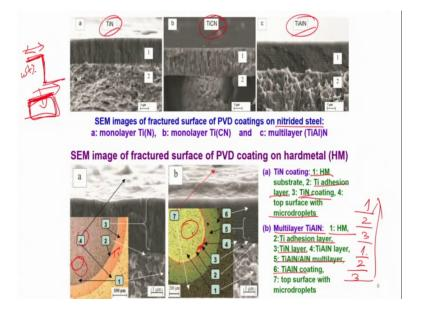
In fact, you can by way of reaction base PVD you can create for example, here you have a nitrided steel and on top of that this is where, in a you have created titanium nitride in b you have created titanium carbon nitride and in c you have created titanium aluminum nitride. So, you have created a single nitride, you can create the carbon nitride, you can create a combined nitride a mixed nitride. And this is possible not just.
