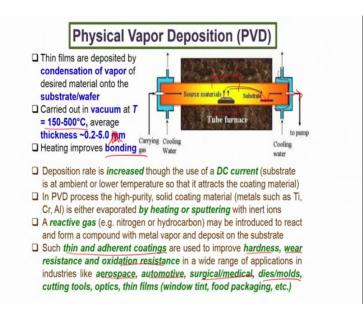
So, you can have instead of enclosing in a chamber like that you can also create of tube furnace like configuration; where, you can keep the holders cooled by flowing air, flowing water through these gaps. You can use these openings to pump out the gas inside evacuate it and this is the source material. And now, you can you heat it in a tube furnace.
