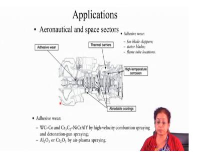
So, now if you particularly go through the application in different sectors, you will find that in aeronautical or space sectors there are major applications of thermal spray deposition technique. They may be applied for adhesive wear applications improval adhesive wear enhance property enhancement, then maybe for thermal barrier property enhancement, they may be for abrasion wear resistance application or high-temperature corrosion application.
