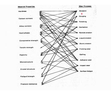
So, now if you quickly go through the different material properties which are required for different wear application you will find that, for abrasive wear application it is very important that the material should have the harder as well as should have a good fracture toughness, fatigue strength should also be quite high. So, where micro structure and composition plays very important role and even different types of wear if you see in different types of wear different properties play role.
