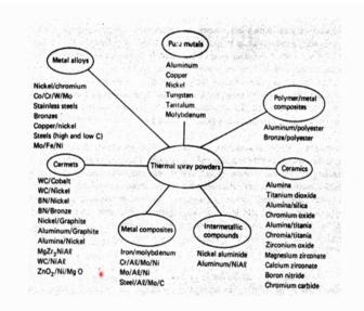
So, whenever you talk about the wear resistance, you can choose the proper material with the desired hardness. Now if you see that different types of materials again, it may be pure metal with different hardness. So, if it is for example, if you are interested to develop a coating which should have very good antifriction property, then you go tin coating as tin coating and pure metal tin you use for coating material.
