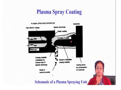
So, a little bit of advancement of these particular technique is the plasma spray coating. So, plasma spray coating is the little bit advancement in the in this stage that in plasma spraying you really get a very high heat into the teep of the torch. So, heat content in flame spraying or arc spraying can be 1500 to 700 degree Celsius, on the other hand in plasma spraying it can be as high as 25000 to 30000 degree Celsius.
