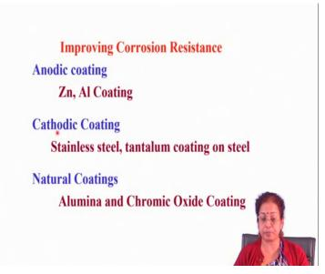
Kinetic spraying can be applied for polymeric coating, can be applied for corrosion resistance application like anodic coating, zinc aluminium, cathodic coating stain less steel, tantalum coating and natural coating like alumina chromium oxide coating.
