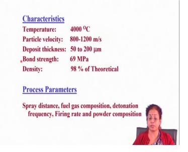
So, as I mentioned you temperature is a quite reasonably good for metallic and metal matrix composite coating. Particle velocity is very high above sound velocity; deposited
