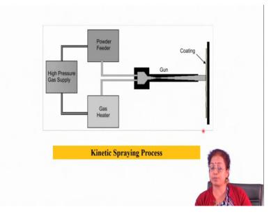
So, the last technique is that kinetic spraying technique where you do not use the heat for spraying operation, but you use basically large kinetic energy for spraying the powder is usually heated because if you do not heat the powder on the powder surface, there is always chance of lot of moisture accumulation moisture absorption.
