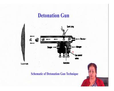
So, another kind of coating is detonation gun coating. So, in detonation gun coating you basically use the spark plasma and you use spark plug for fuel for a ignition of the fuel. So, what you do is that, here actually instead of having the torch for fuel ignition you can have the local localised zone for ignition of the fuel and hence heat generation.
