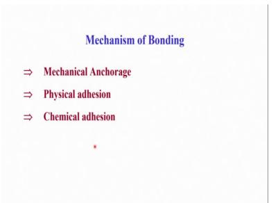
Now we quickly go through the mechanism of bonding in thermal spray deposition, these are mechanical anchorage physical adhesion as well as chemical adhesion. So, mechanical anchorage is always they will show accordingly for all the processes so, you have to prepare the substrate so, that there are lot of roofs on the surface we usually do it by sandblasting operation.
