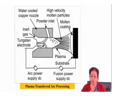
So, another type of you can say that little bit closer to quelling process is plasma transferred arc processing. So, where basically the arc process though the electrical arc current passes though the plasma and then it strikes the substrate surface. So, plasma is very close to the substrate because of its closelyness in nature, you will find that molten material get deposited over the surface of the substrate like way lowerly.
