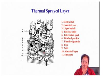
Now, if you quickly go through the thermal sprayed deposited layer cross section, you will find that as I mentioned you in the last few slides that there are lot of defects in the coated layer like oxide particle inclusive small small unmelted particles and then the parts are basically a they are in the form of the this molten material are in the forms of spalt.
