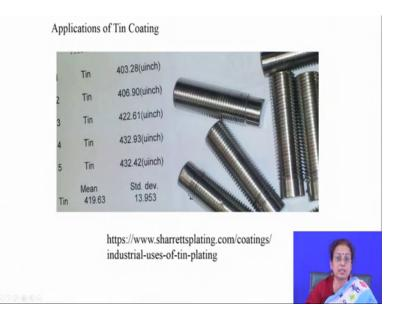
These are some of the applications where thin coating has been applied for that typical food containers which is where you will find that the coating looks coating surface looks highly glazy and back appearance, you can also have the screws and then big beverage containers coated with tin.
