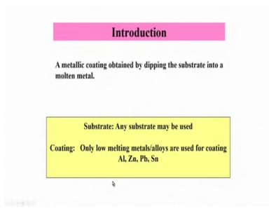
As their name implies this is here hot dipping this is nothing, but a kind of technique or may be series of techniques which are applied for development of metallic coating and obtained by dipping the substrate into the molten material which you are going to deposit. And usually the substrate may be anything, but should have very high melting temperature and the coating should have quite low melting temperature.
