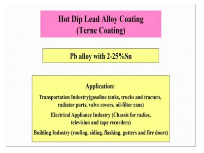
And so these are the parallel techniques, so another alloy which is basically used for a hot dipping operation is nothing, but terne coating that is again lead alloy with 2 to 25 percent tin. So, this is lead based alloy, so and this is lead based alloys, so basic purposes mainly for improving the anti friction property and tin is quite high. So, tin has to be used because the otherwise lead is having very poor wettability.
