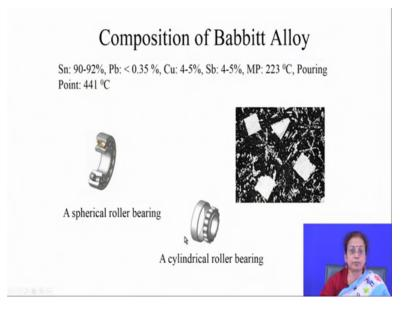
So, these are different bearings coated with thin lead alloy that difficulty babbitting babbitt alloys. So, as I mentioned you that typical compositions have a little bit of plate, so this is typical 90 to 92 percent tin less than 0.35 percent lead, copper 4 to 5 percent, antimony 4 to 5 percent, melting point is quite low 225 degree Celsius and pouring point naturally 441 degrees Celsius much higher than that of melting point.
