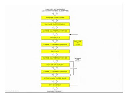
So, similarly tin coating also if you talk about parallel techniques; parallel techniques are for example, electro deposition of tin. So, electro deposition is also often applied and prefer to hot dipping process because after hot dipping you have to go for machining operation as they are hot dip layer is basically the molten and cast layer more melt and cast layer. So, this is having lot of a roughness surface finish is not so good, so you have to go for the finishing operation.
