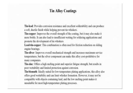
So, apart from this tin is used in pure form for different applications as I mentioned you can be used for corrosion resistance aqueous corrosion resistance application as cans and cans for food and beverages, can also be used for anti friction property enhancement, it can also be used for typical soldering as a base for soldering application.
