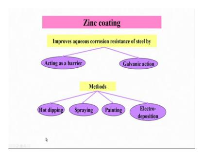
And finally, the biggest industry of hot dipping is for zinc coating, so you got to tell it as hot dip galvanizing. So, zinc coating basically zinc coating is very much applied for protecting against the corrosion resistance.
