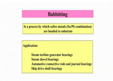
So, next I will discuss about babbitting technique which is nothing, but again tin based alloy. So, there are different babbitting alloys which are applied, but the basic purpose of babbitting is that not really to improve the corrosion resistance because usually you use lead in this tin alloy and when lead present naturally it is not really non toxic as pure tin and its corrosion resistance also decreases to a little extent.
