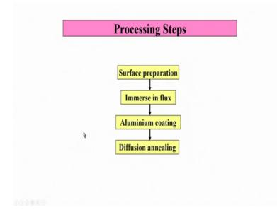
So, this is about the one step process and in two step process what you do is that you prepare the surface and then you immerse it in flux molten flux, then you go for this particular deposition dipping operation and then go for the final annealing. So, these are there two different processes. So, one step processes are having certain advantage, one step process is having several advantages like this is very quick process.
