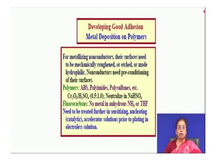
And usually nonmetallic materials are deposited by electroless deposition. So, this is very useful technique for and also a kind of important technique to deposit a very thin deposited layer by electrodeposition where the substrate is non conductive.
