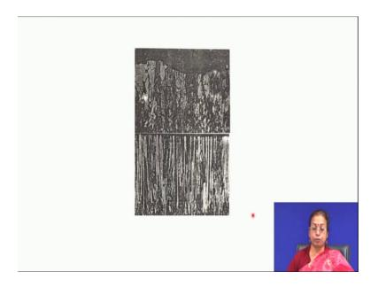
Usually, if you talk about dc electro deposition process, there you get very large columnar grains or density grains. On the other hand if you talk about the electro deposition where pulse a pulse reverse mode, your deposition structure is highly uniform it is compact in nature.
