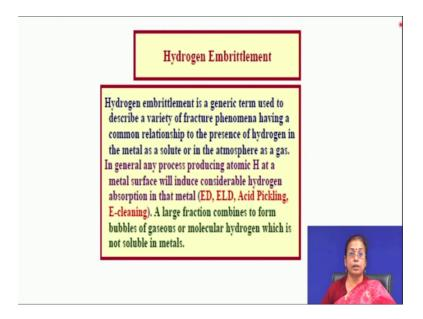
So, one of the important process which is which plays very important role in electrodeposition is that evolution of hydrogen actually. So, hydrogen evolution is a competitive process. So, in the cathode there is hydrogen evolution as well. So, whenever you talk about electrodeposition or electroless deposition, naturally atomic hydrogen they are basically they may get diffused in.
