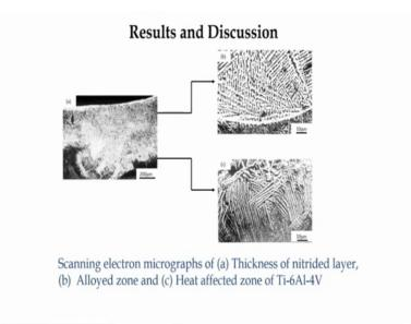
If you see the surface carefully you will find that there is lot of dendrites containing the nitrides titanium nitrides and also the continuous and monolithic continuous and defect free solid liquid the interface where nothing was present, as it was melted with laser beam the heat affected zone was also negligible in nature
