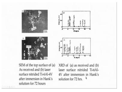
And interestingly again this particular nitriding operation was also aimed at improving the bio activity of titanium surface. So, we try to see the bio activity behavior by immersing it in Hank's solution and subsequently measuring the calcium phosphate deposition rate regular interval.
