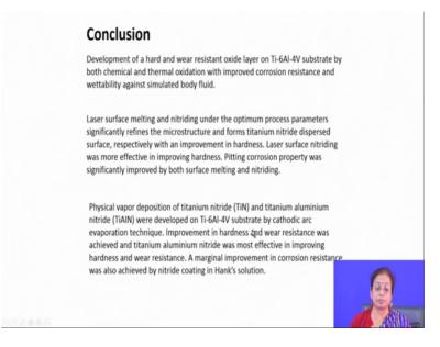
So, it can be concluded that the oxide layer, nitride layer may be I mean oxide layers on the surface of metallic materials may be developed by chemical oxidation route, may be developed by thermal oxidation routes, may be developed by typical laser processing route and is very much applicable treatment for improving the corrosion resistance as well as wear resistance of the surface.
