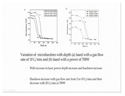
So, you find that as we go on increasing the power you will find that there is decrease in hardness because of the increase inter dendritic spacing. On the other hand if you just go on here, in this case we also had the shrouding environment pressure as another variable.
