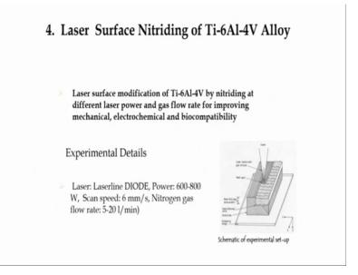
Now, another way by which you can also convert the surface of metallic materials to its nitride or oxide is by melting and subsequent just subsequent application of that reactive stout. For example: the surface nitriding is one such example where it has have it is a lot of examples on the titanium as well as a steel substrate where you can melt the surface using the high power laser beam and then use nitrogen stout, so that there is formation of nitride layer on the surface.
