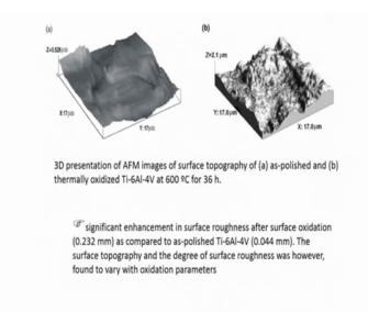
So, because of oxidation there was naturally improvement in the increase in surface roughness. So, that surface roughness enhancement was beneficial because if you have the increase surface roughness, it basically promotes a cell osseointegration and cell growth on the surface.
