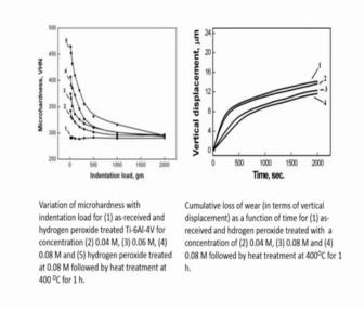
So, we will find here accordingly the micro hardness also changes because of formation of anodized field, you will find that there is improvement in hardness and depth of the hardening was around 10 to 15 micron.
