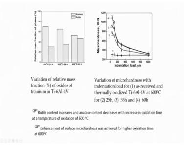
And as a result of which we found that there is improving improvement in hardness and if you just compare the hardness enhancement with respect to that of chemically oxidized layer you will find that it is 4 to 0.5 times higher than that of chemically oxidized converted titanium dioxide.
