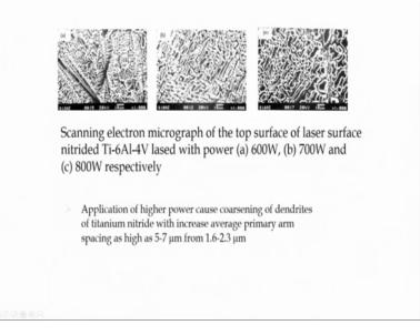
So, it was observed that as you go on increasing their power this particular thickness of the that area fraction of the dendrites increases as well as you can say that here dendrites are basically mostly very long dendrites in nature particularly when your temperature or that power of laser is very high. On the other hand whenever it is very low you will find that dendrite count spacing is quite low because of very high cooling rate.
