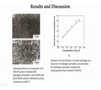
And this oxide was mainly and it is in nature and if you see the oxide scale properly you will find that the oxides are very much very fine oxides are present. And, if you see the morphology it you will find that very nano very thin fine nano cells precipitations are observed on to the surface and as you go on increasing the hydrogen peroxide concentration you will find that area fraction of the particles also increases.
