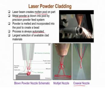
So, as I just now said that you create a molten pool, you can blow powder into the molten pool or a feed a wire into the powder pool powder pool and melt pool, and the whole process can be automated and you actually can have a very large selection of materials varieties of materials.
