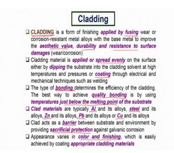
So, as I said overlay is very popularly called cladding because you actually are creating a new layer on top of that. And this is created by fusing wear or corrosion resistant metals or alloys with the base metal, and we can improve the aesthetics of the substrate, the durability the resistance to surface dependent damages like wear or corrosion and so on.
