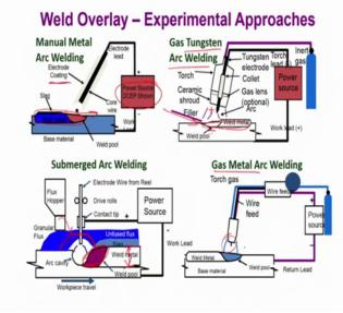
Now, typical processes particularly on the arc based process, which are very popular because of productivity, because of versatility and also because of the ease with which one can actually use for various kinds of materials. So, one of the most common and conventional method is called manual metal arc welding. So, manual essentially means that actually you have an operator who actually holds the torch which actually the electrode one of the electrodes.
