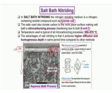
So, typically when we talk of liquid nitriding then we use the cyanide as the precursor and when we stock of salt bath nitriding then we can directly use the sodium cyanide salt. And these sodium cyanide salts at that high temperature dissociate.
