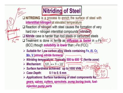
So, today we are going to discuss a nitriding of steel and in particular Gas Nitriding. So, first of all as I said nitriding essentially means we are going to enrich the surface of steel with the nitrogen and obviously, nitrogen is one of those four elements which are fairly small to be able to find a place in the interstitials of alpha iron or a BCC iron. For example, we all know that a hydrogen, carbon, nitrogen and oxygen are the elements which easily can be accumulated in the interstitials
