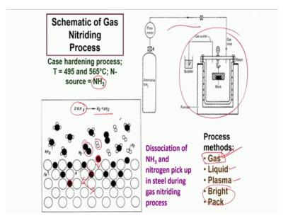
So, we must realize that though the source is a ammonia at high temperature should dissociate and provide nitrogen and hydrogen molecules, but the molecular form is not fit enough to enter into the lattice. So, they need to so, if you have an N 2 or H 2 molecule they actually need to further dissociate and reached the nascent state. So, that now this nitrogen atom is in a position to get adsorbed onto the surface layer and subsequently can actually diffuse likewise in this path.
