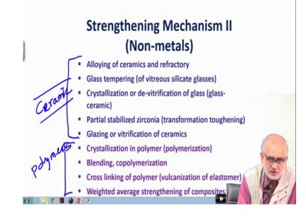
So, we will be discussing for example, a large extent on the ceramic materials. So, these are the various ceramic strengthening mechanisms applicable to ceramic materials, we will also be scribing the strengthening mechanisms applicable to polymers.
