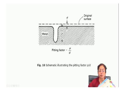
So, it is also evaluated by pitting factor; pitting factor is nothing, but if the rate is the ratio of overall pit depth total pit depth and also pit depth to the overall corrosion. So, whenever there is pitting at a naturally there is also normal (Refer Time: 04:56) corrosion factor because metal whenever you exposed to the environment naturally there will be general corrosion as well as pitting corrosion.
