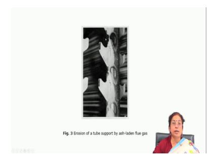
So, erosion corrosion of that you suffered by ash laden flue gas you see erosion corrosion can be so, high that it cause the damage at the corner point.
