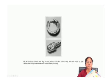
Similarly, if you are interested to reduce it you can hard face it for example, hard face stainless steel plug and seat it is again a kind of though hard face, but you see that there is also erosion corrosion by high velocity flow through a narrow or if is created during that typical throttling operation. So, you will find that because of that a very large amount of energy is associated with that flow and it causes the damage of the component.
