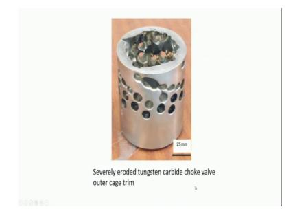
They severely eroded tungsten carbide choke valve outer cage trim, so you see how badly it has been affected. So, big cavity formation are there all throughout the surface of this metal component. (Refer Slide Time: 27:34)
