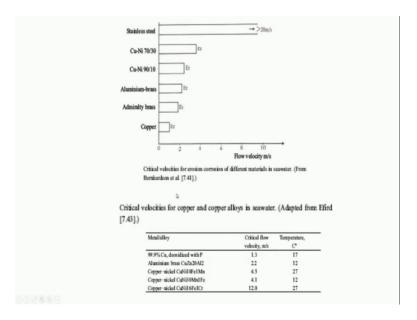
Now, it is very important to know at which velocity the pitting corrosion will (Refer Time: 17:47) that crevice corrosion that erosion corrosion will start because if you are interested to choose the material for your choice, then naturally for the component of your choice naturally you have to choose it properly. So, that it does not get eroded in the particular environment or in that particular flowing environment.
