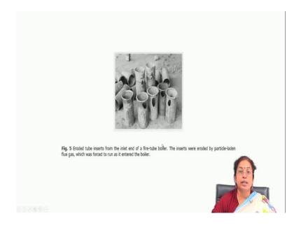
The example of eroded tube inserts from the inlet end of fire tube boiler, the inserts were eroded by particle added flow gas which was forced to run as it basically enters the boiler.
