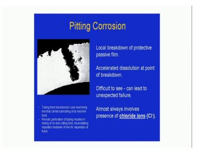
Now, if you talk about pitting corrosion this is also a kind of localized form of corrosion which looks like pitted on the surface. So, after this corrosion you will find that there is pit formation on the surface and the driving for the particular pitting corrosion is nothing, but again local breakdown of the protective passive film and subsequently galvanic cell formation between the expose surface and also the protective surface.
