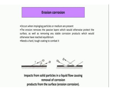
Now, next type of corrosion which is very important is that erosion corrosion. So, pitting corrosion and crevice corrosion their more or less similar in nature here the initiation mechanism is by micro galvanic cathode. But if you talk about erosion corrosion it is a little different in nature here also there is chance of the that particular breakage of that surface protective film, but because of the action of erosion.
