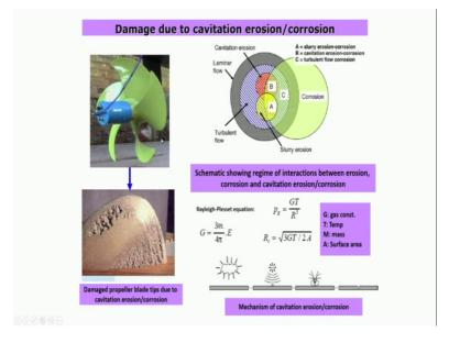
Now, one typical kind of for very interesting example of erosion corrosion is the cavitation erosion phenomena. So, normally erosion corrosion is usually observed in the constructed part its sea water or flowing in component in the sea water particularly if we just talk about the marine component that water pipeline or may be in the case of oil and gas pipeline you will find the erosion corrosion is very much prominent, its sea follows erosion corrosion is very much applied.
