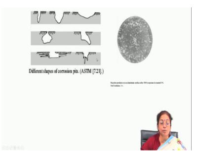
Now, if you quickly go throw the pitted surface on the surface it appears likes small small pits having different dimensions, starting from micrometre starting from nanometer to micrometer to macrometer level. And if you just quickly go through the depth or it how it propagates how does it look like along that you will find that, along depth sometimes it is tubular in nature, sometimes it is regular in nature, sometimes it is zigzag need process in a zigzag fashion.
