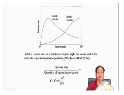
So, erosion corrosion is very much dependent on the not only that surface hardness and microstructure, but also depends on the impeachment angle. So, the flow if flow direction plays a for example, when the component is expose in natural environment in water, in pond or in case of river or in case of sea you will find that rate of attack is very much dependent on the direction of flow.
