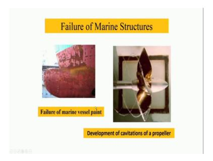
Few examples of cavitation corrosion includes, the failure of marine vessel paint, development of cavitations of a popular.
