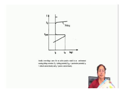
So, this particular pitting corrosion rate as I mentioned you that if you are interested to evaluate the pitting corrosion you have to know the area fraction of the porosity to a large extent with the help of typical microstructure analysis, otherwise you can also measure the pitting corrosion rate by electrochemical means.
