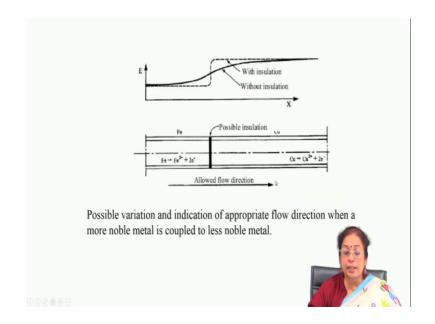
So, this is again flow (Refer Time: 14:05) again the combinations for iron and copper. So, you will find that if you go on insulating the part naturally you can minimize the tendency of the attack of the typical anodic part of the combinations of the couple.
