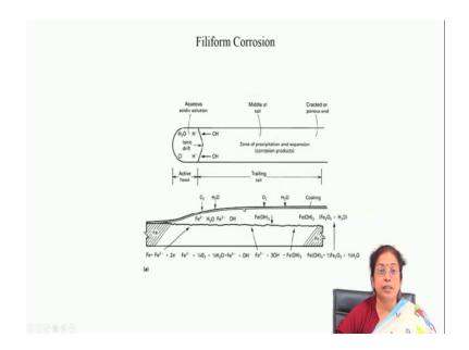
So, one of the important form of crevice corrosion is filiform corrosion which usually is observed in the painted surface. So, what happens is there in the painted surface? There is always very small small nano level perforations or porosity is micro to micro level porosity is to nano level porosities.
