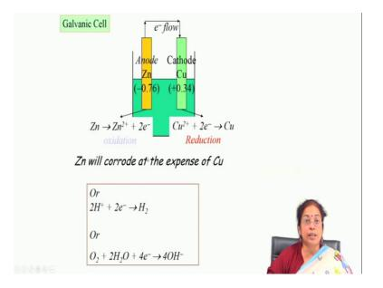
So, this is the case for the zinc and copper whenever you immerse it in typical hydrochloric acid solution you will find that and if you have connect them properly you will find that the zinc corrodes and at the expense of copper. So, copper is actually protected, but zinc goes on corroding to a large extent. So, this is typical galvanic cell.
