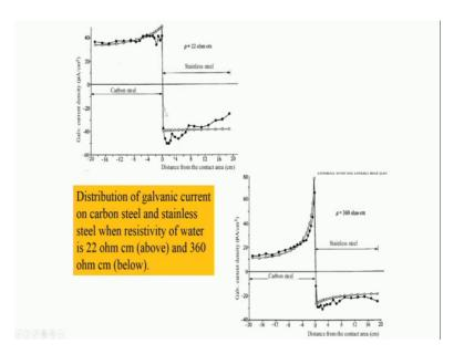
This is the case for carbon steel stainless combinations, it also depends on you will find that carbon steel that this particular galvanic corrosion current density is much higher than that of stainless steel which is says basically non corroding in nature. And it also depends on the resistivity of the environment solution particularly.
