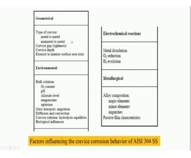
So, if you just quickly go through their different factors or parameters which influence the crevice attack of a component, these are apples. For example, that type of crevice whether it is metal to metal combinations or non metal to metal combinations. The gap and degree of tightness, the crevice depth, then exterior to interior surface area ratio.
