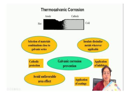
The this is the case for thermogalvanic corrosion where you find that hot part actually acts as anode as compared to that of cold part and problem starts at the interface. Now, if you quickly go through the way by which you can compare the galvanic corrosion.
