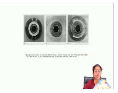
Then crevice related corrosion for different alloys in natural sea water again you will find that lot of corrosion is there at the crevice site as compared to that of our surrounding region.
