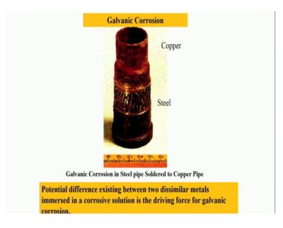
So, galvanic corrosion is a form of corrosion which usually occurs when two dissimilar metallic materials are electrically connected and they are placed in an aqueous media or electrolyte. So, usually the potential difference existing between the two dissimilar materials is a driving force for the corrosion to occur.
