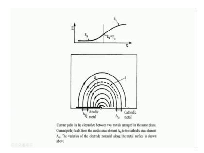
So, current part in the electrolyte between two metals for example, if you have that anodic metal and then cathodic metal, so you will find that naturally the problem starts at the interface. So, the that anodic side basically corrodes to a large extent and by that process it protects the surface of the cathodic metals.
