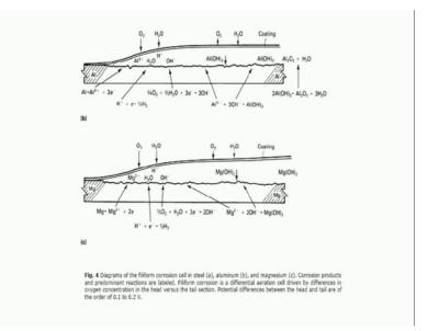
So, when you look at the surface you will find that it basically the filiform for filiform corrosion basically, the appearance of the filiform formation is like in a tubular fashion zigzag zone on the surface.
