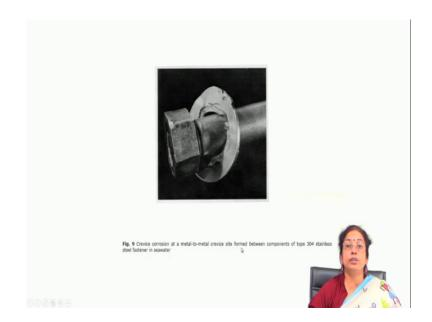
So, you have to be very much careful and design the component combinations properly, so that you can compare that possibility of the crevice attack. This is the example of crevice corrosion at a metal to metal crevice site font between the components of type 304 stainless steel fastener in seawater. So, you find that lot of crevice corrosion is there at the in the fastener.
