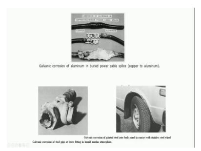
So, naturally you will see that usually that the interface plays is a very important role and everything, every problem starts from the interface. This is the galvanic corrosion of aluminium and copper coupling as I mentioned you, again galvanic corrosion of painted steel body steel auto body. So, you will find that there is by some way by erosion corrosion or by the typically the exposure of this particular painted surface to environment.
