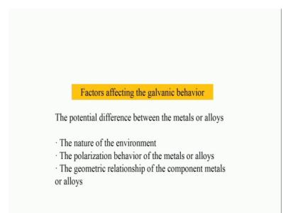
Now, the factors which influence the galvanic behavior there ample for example, the potential difference between metals and alloys, so how they are basically placed in the galvanic series. Second part which is very important is that the kind of environment the component is exposed to because defending on the environment again, the position of different material or chemically reactive nation of different metal changes.
