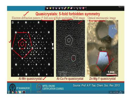
So, I must show you some of this pattern electron diffraction pattern of quasicrystal and the in the left hand side this is an image that is taken from a 5 fold, and this is an aluminum magnesium quasicrystal and you can see here very interesting thing. So, I show you here 1 regular pentagon here you can see and now here is another pentagon.
