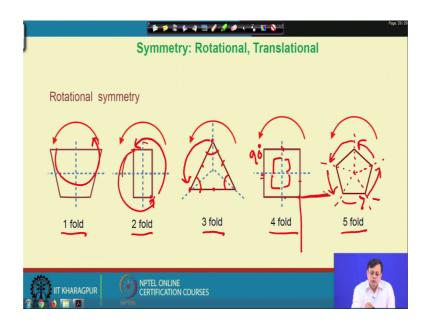
So, 360 degree rotation it require and therefore, we call it as a 1 fold symmetry. Now in this case let us say a rectangle let us say, we can see these are some of the symmetry axes and if we rotate it 180° then this point will come here and definitely we will get a 2 fold. So, means this point will come from here to here and then we make another fold. So, that this point will come back to it is original position ok.
