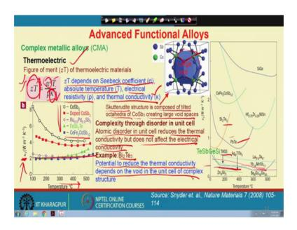
The other uniqueness of such complex alloy phases are the thermoelectric material. Usually for thermoelectric material a figure of merit that is represented by zT is the alpha square T by rho into K; here zT depends on the Seebeck coefficient alpha and absolute temperature T and electrical resistivity rho and the thermal conductivity.
