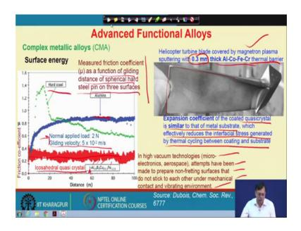
Now, due to such surface energy differences we think about the friction coefficient of such CMA. And I show you another example use of such icosahedral quasi crystal which is a i phase we call it as a aluminum and copper iron and boron phases; which has the lowest friction coefficient compared to alumina or hard steel. So, this is a stress that is applied at 2 Newton with a gliding velocity of 5 into 10 to the power minus 2 meter per second.
