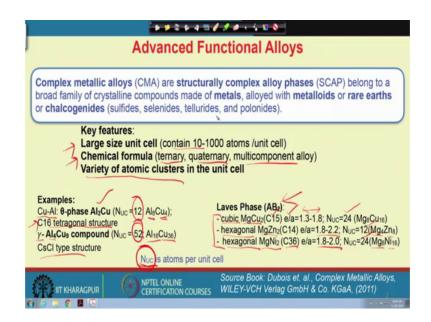
These complex metallic alloys are structurally complex alloy phases belong to a broad family of crystalline compound made of metals, alloyed with metalloids, rare earths and chalcogenides. So, chalcogenides means let us say tellurides, sulfides, selenides, polonides and so on. So, from this basic definition we can easily try to understand that these must be very close like inter metallics, but having very complex structures.
