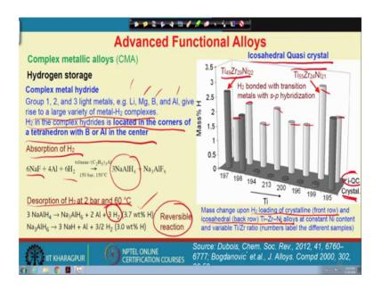
Now, another example is the hydrogen storage. So, usually for hydrogen storage complex metal hydrides are often used and these are basically the group 1, 2 or 3 light elements like you have lithium or magnesium or boron aluminum that gives rise to a large variety of metal hydride complexes and this hydrogen is a complex hydride located at the corner of a tetrahedron with boron or aluminum at the centre.
