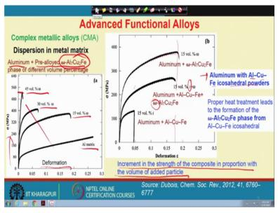
Very similar way another example of such dispersion in metal matrix I show you here in case of aluminum and pre alloyed omega phase. So, this is also a complex phase which has been reinforced in a aluminum matrix, this is the strength versus ductility you can see with increase of the omega phase the ductility decreases whereas, the strength is increases.
