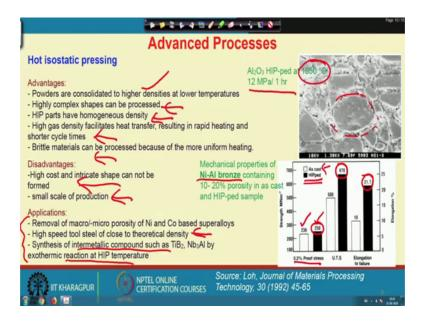
Now, the advantage and disadvantage of this hot isostatic pressing is like here the powders are consolidated at a much higher density and much lower temperature that I have already shown you in my earlier slide.
