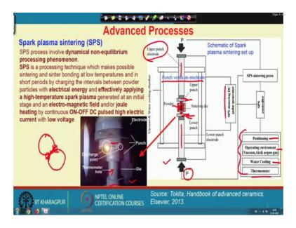
Now, for spark plasma sintering SPS process involve a dynamical non equilibrium processing phenomena; means, so the SPS processing technique which is possible sintering or sintered bonding at relatively lower temperature and in a very short period.
