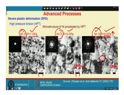
I show you a just 3 example of such microstructure. Here this is number of turn is 5, here also number of turn is 5, but the effect of pressure it is 1 Giga Pascal, 3 Giga Pascal and 9 Giga Pascal during high pressure torsion. So, the scale bar here is 1 micrometer, 0.2 micrometer means, 200 nanometer and here this is 100 nanometer. You can see that by application of a higher pressure, we can easily reach to a nano scale grain by the same number of turn by increasing the applied pressure.
