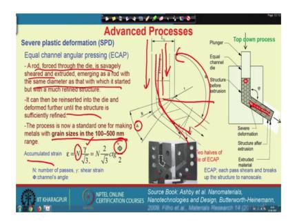
So, I can show you some of the schematic of such a SPD process and you can see that by simply pressing through a SPD process like a ECAP, the material is pressed through that. And we have a angle that is let us say psi and so the accumulated strain that is the number of the passes and the strain shear strain that we introduce divided by root over of the 3 and that is also linked with how much angle we provide.
