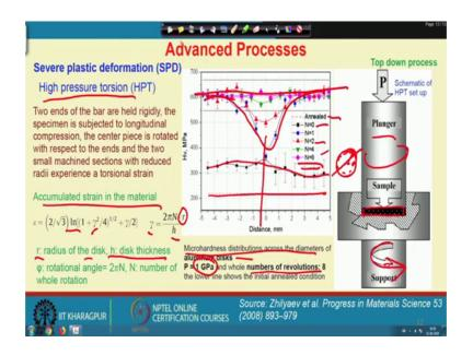
Now, the second severe plastic deformation process is the high pressure torsion, in that particular technique the two ends of a bar, so here there are 2 plunger and we have the sample here and we rotate this plunger in the opposite direction ok. So, if I have a disc then at the circumferential region I will introduce maximum amount of strain because, the more strain is achieved at the r theta.
