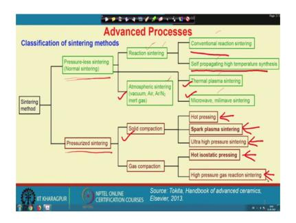
So, if we look at the scaling up process and sintering is one of such process where, we start with powder and we make bulk solid out of it. So, there are 2 major type of sintering are possible, one is pressure less sintering; that is a conventional sintering process, whereas there are pressurized sintering means, during sintering process we apply pressure.
