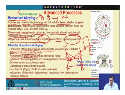
Means I can have copper, I can have nickel individual particles and by this mechanical alloying technique, we can make a alloy of nickel and copper.
