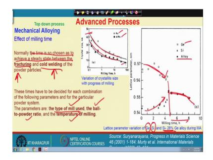
Now, the time is also very much important ok. So, how much time you will allow for a milling purpose. So, like a crystal size here I am talking about the in maybe the particle is self is one micrometer, but inside a particle there are many crystals ok. So, those crystals size can be easily measured using X ray diffraction and we call it not as a crystal, it is a crystallite size ok. So, means the individual domain, that contribute to the diffraction.
