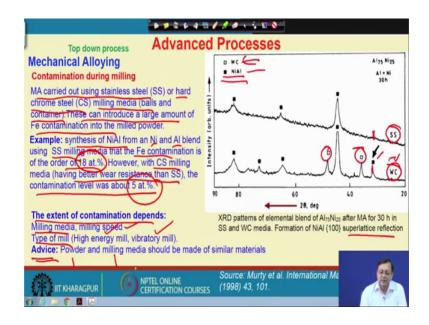
Now, besides all these processing parameter, one important aspect one has to keep in mind on processing these advanced materials using these non equilibrium processes like mechanical alloying that is basically, the contamination. You are milling or we are milling in a medium using a vial and the ball. So, the vial and the ball they may also add some contamination and change the purity level of the powders that you are going to produce.
