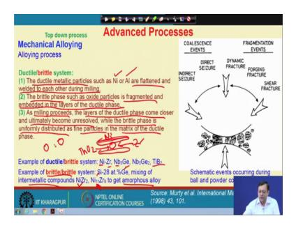
However, the system mechanism may altered when we consider a ductile brittle system means, one of the initial particle is very hard and another one is relatively soft.
