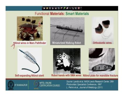
Now, there are huge number of application of such smart metal or shape memory nitinol alloy, there are many alloys has been developed. So, let us have a look, so like the Nitinol wires, which was used in Mars Pathfinder, and for using some antenna, which open and closed due to temperature variation or even you can put some of this antenna in the polar region, where there is temperature gradient or there is a huge thunder storm goes on and so on.
